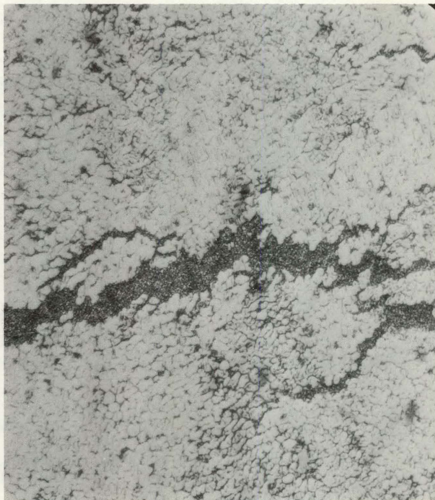
Figure 6. PHOTOMICROGRAPH OF THE STEP AREA SHOWN IN FIGURE 5. (Again, Microcracks have been Backfilled with Al/Be Eutectic; As Polished; Bright Field Illumination; 750X)
