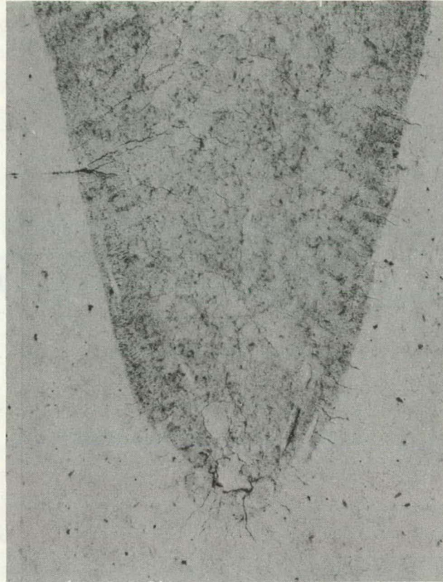
M383-5b Figure 3. PHOTOMICROGRAPH OF THE WELD FROM RING 3A, AT THE 180-DEGREE LOCATION. (The Prior Microcracking is Very Evident at the Step and Root of the Weld; As Polished; Bright Field Illumination; 75X)
