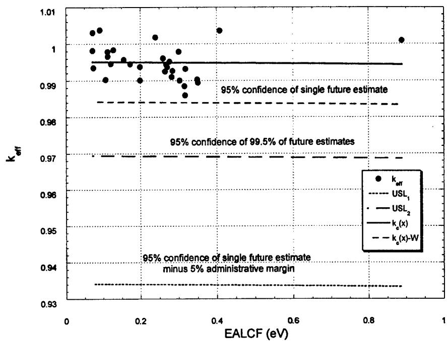
**Figure 1.** Scatter plot  $k_{\text{eff}}$  vs. EALCF for 238-group ENDF/B-V library.
