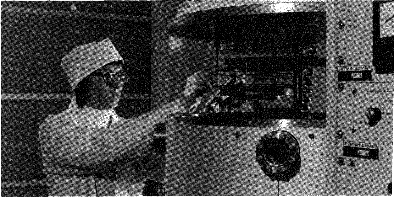
Sputtered tungsten provides long life electrical connection for the RTG thermopile.
