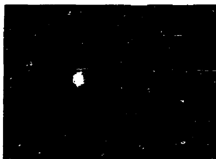
Fig. 9. Electron beam profile of a poorly steered beam. Large tails are evident.
