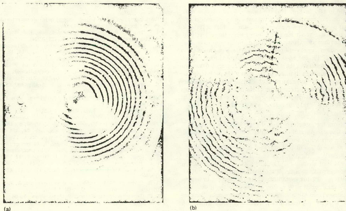
FIG. 2. Holographic interferograms of the rear surface of an aluminum plate of thickness 0.635 cm and diameter 5.08 cm at (a) 0.92 \mu sec and (b) 1.02 \mu sec after energy deposition. The scribe marks are 0.508 cm apart.
