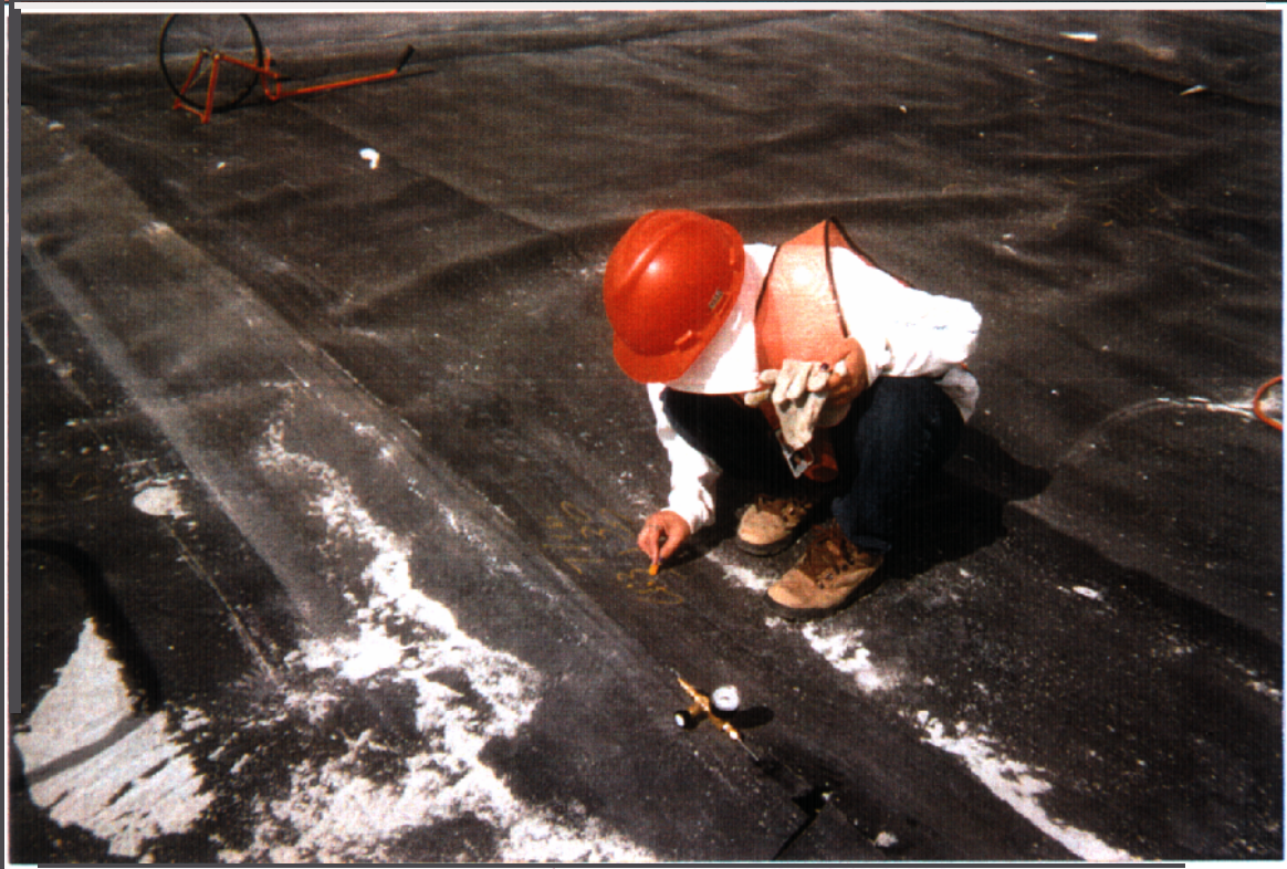
Photo 9: Air-pressure testing of fusion seams. Technician writing results on liner.
