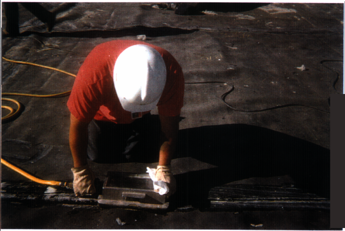
Photo 10: Non-destructively testing extrusion weld with a vacuum box.
