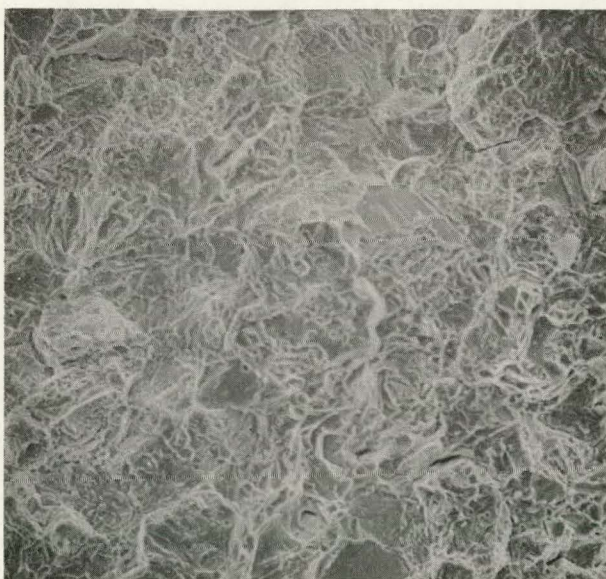
FIGURE 6. Mixed Fracture of Single-Edge-Notched Specimen Tested at 78 K
