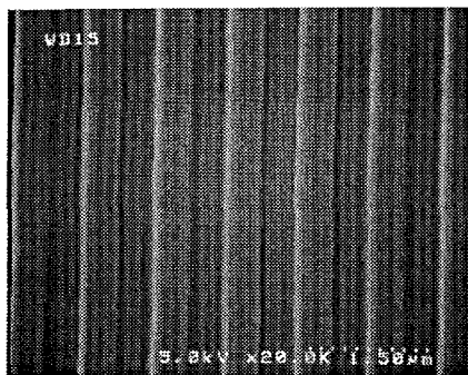
Figure 4. Reflective grating mask imaged by Schwarzschild camera into SAL 603 resist.
