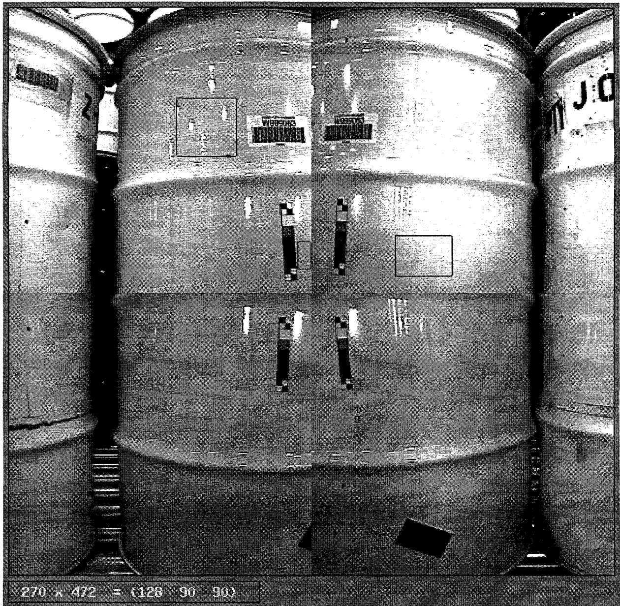
Figure 6-4. Image of a defective drum displayed from within the Mission Assessment screen of the IMSS operator interface.
