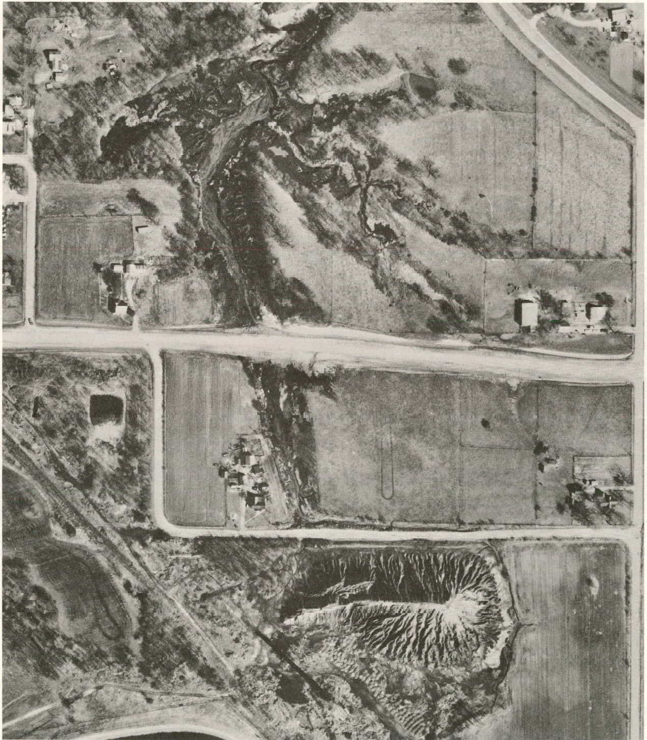
Fig. 2. The Staunton 1 site before reclamation. The gob pile is at the lower right, and drainage from the pile flows northward to the dark slurry area at the upper center.
