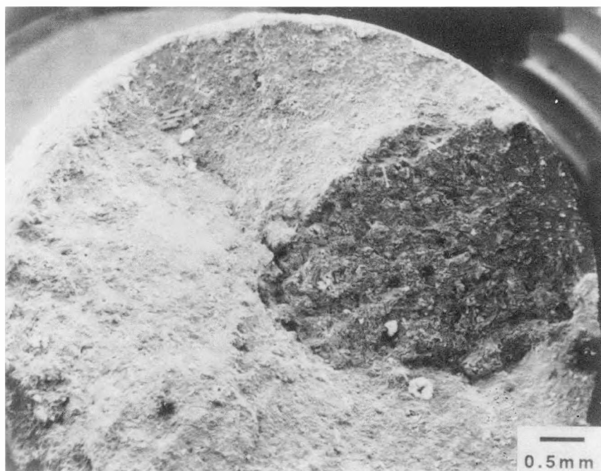
Figure 24. Fracture Surface of A106B Ferritic Steel (Heat No. DP2-F30, Specimen No. 30C-1) after a CERT Test in Water with 0.2–0.3 ppm Oxygen at 289°C. Transgranular cracking is evident.
