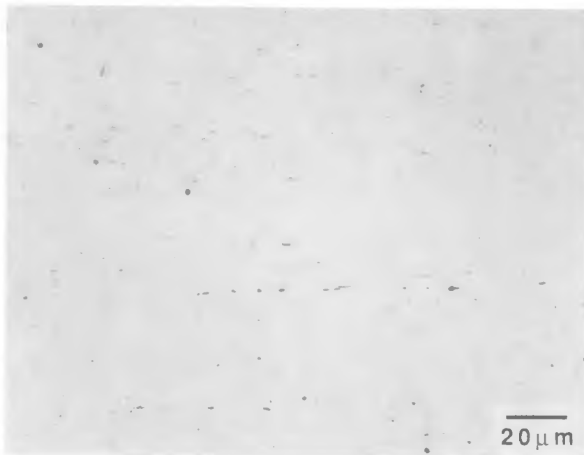
Figure 26. Longitudinal Cross Section of A106B Ferritic Steel (Heat No. DP2-F30, Specimen No. 30C-1) Showing Distribution of Inclusions.
