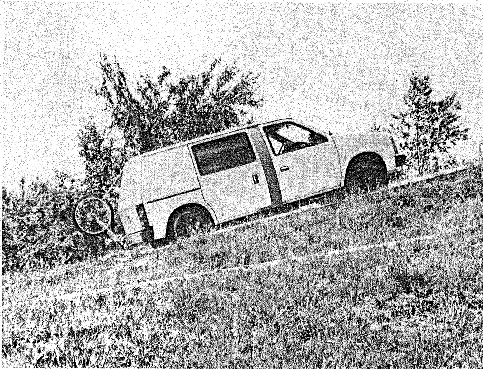
Figure 6 TB-1 Vehicle Gradeability Test
