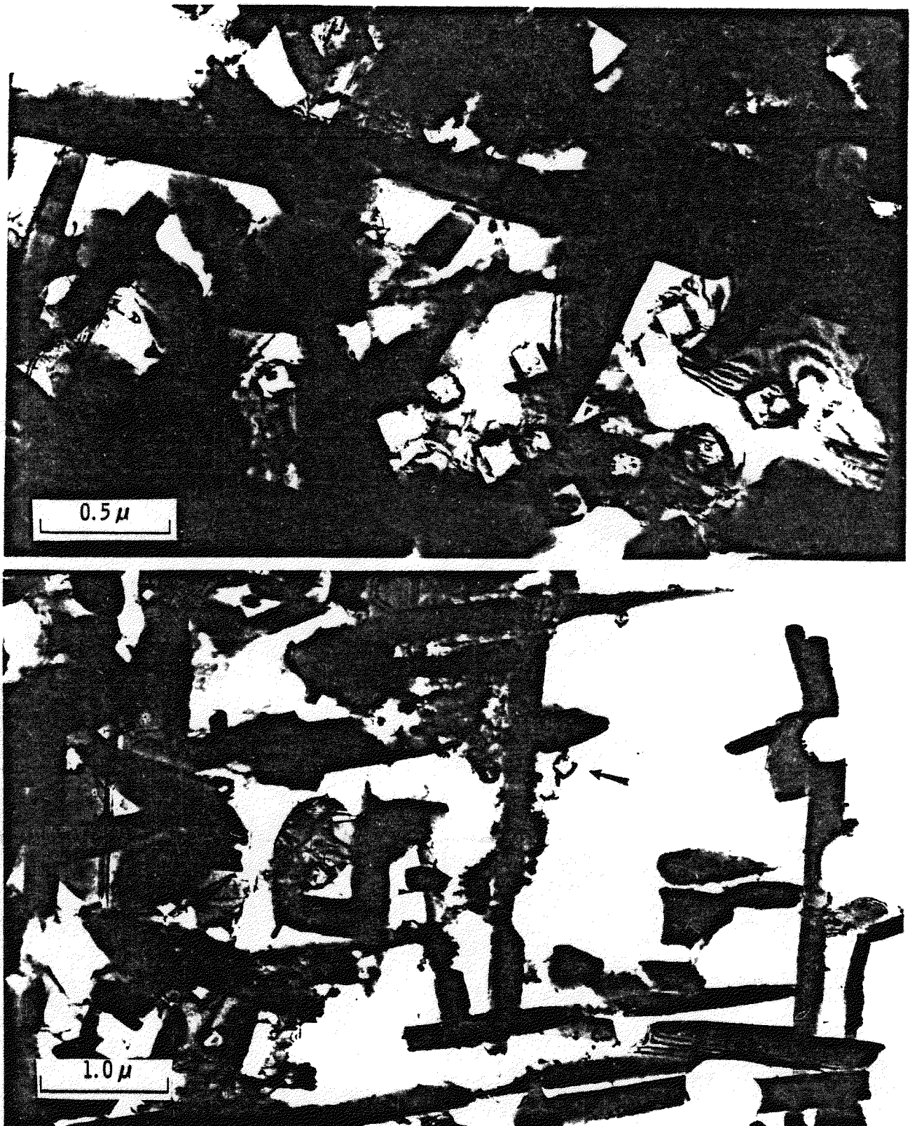
Figure 4. Micrographs showing formation of large iron-rich ferrite precipitates protruding from the strongly etched austenite matrix in Fe-5Cr-15Mn at 520°C and 14 dpa. Voids are also coated with ferrite and resist electropolishing. The arrow in (b) points to an almost unsupported void which has resisted electropolishing.
