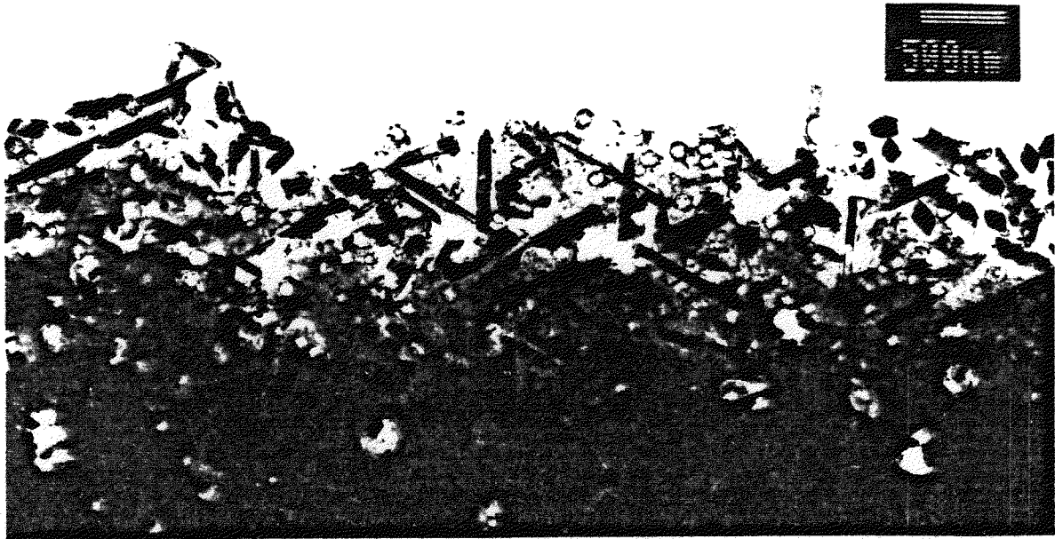
Figure 5. Decomposition of Fe-35Mn at 520°C and 14 dpa.
