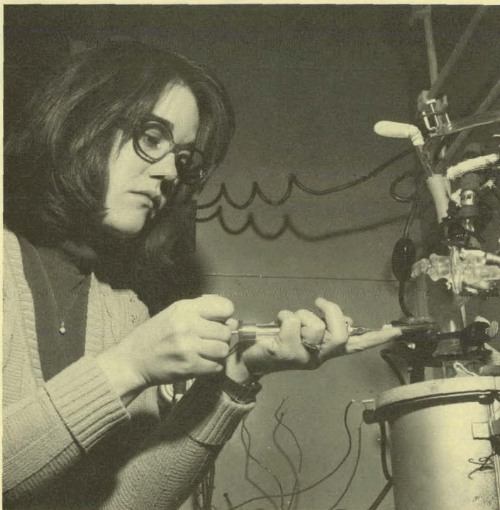
Virginia Morris draws a gas sample produced by heated grain dust. The apparatus is a specially designed tube furnace built in the Glass Shop.
