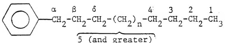
terminal  $\text{CH}_3$ ), respectively. Signals at  $\delta$  37.3, 31.9 and 30.0 could be assigned to carbons  $\alpha$ ,  $\beta$ , and  $\delta$  to an arene ring, respectively. It is also possible that these latter signals could be partially explained by
