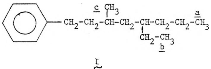
methyl groups (b and c) and a main side chain terminating in a single methyl group (a). Ignoring the possibility of naphthenic material for the moment, one can see that if the relative amounts of  $\alpha\text{-H}(\alpha$  to Ar) and term  $\text{CH}_3$  can be determined and, making the assumptions stated previously, one can calculate the apparent branching per side chain as follows:
