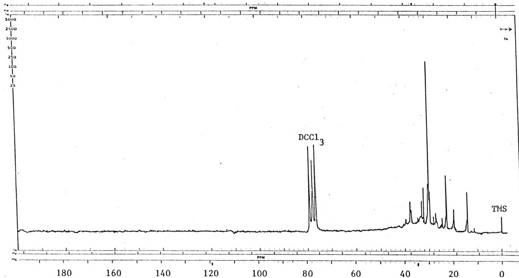
Gated Decoupled (off delay) Sample contained 0.05 M  $\text{Cr}(\text{acac})_3$
