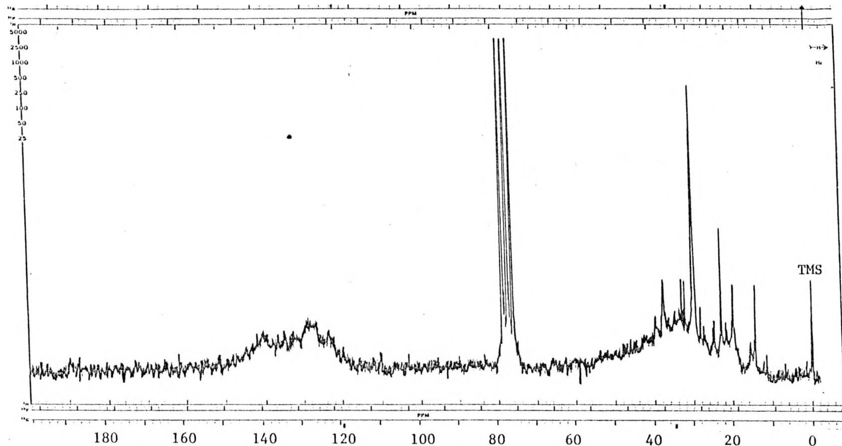
Gated Decouple (off delay) Sample contained 0.03 M  $\text{Cr}(\text{acac})_3$
