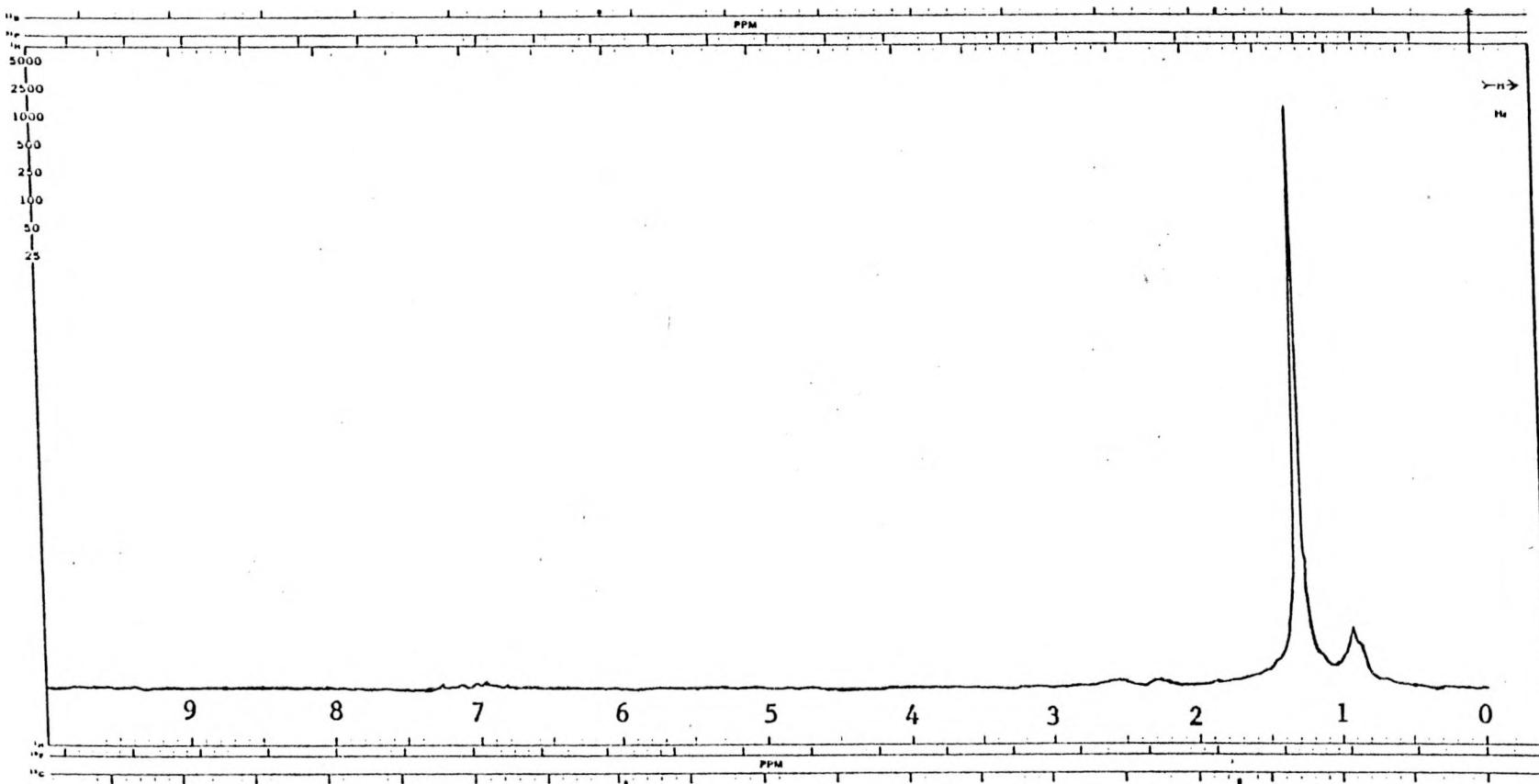
PFT X CW \_; Solvent. .  $\text{DCCl}_3$  ; S.F. . 100.1 Hz; P.W. . 1000 Hz; F.B. .  $\pm$  700 Hz; Acq/S.A. . 64 D5/S.T. . 2.0 s; S.O. . 45251 Hz; T. . 37 °C; P2/RF. . 5.7  $\mu\text{s}/\text{dB}$ ; Size. . 8 K; Lock. .  $^2\text{H}$
