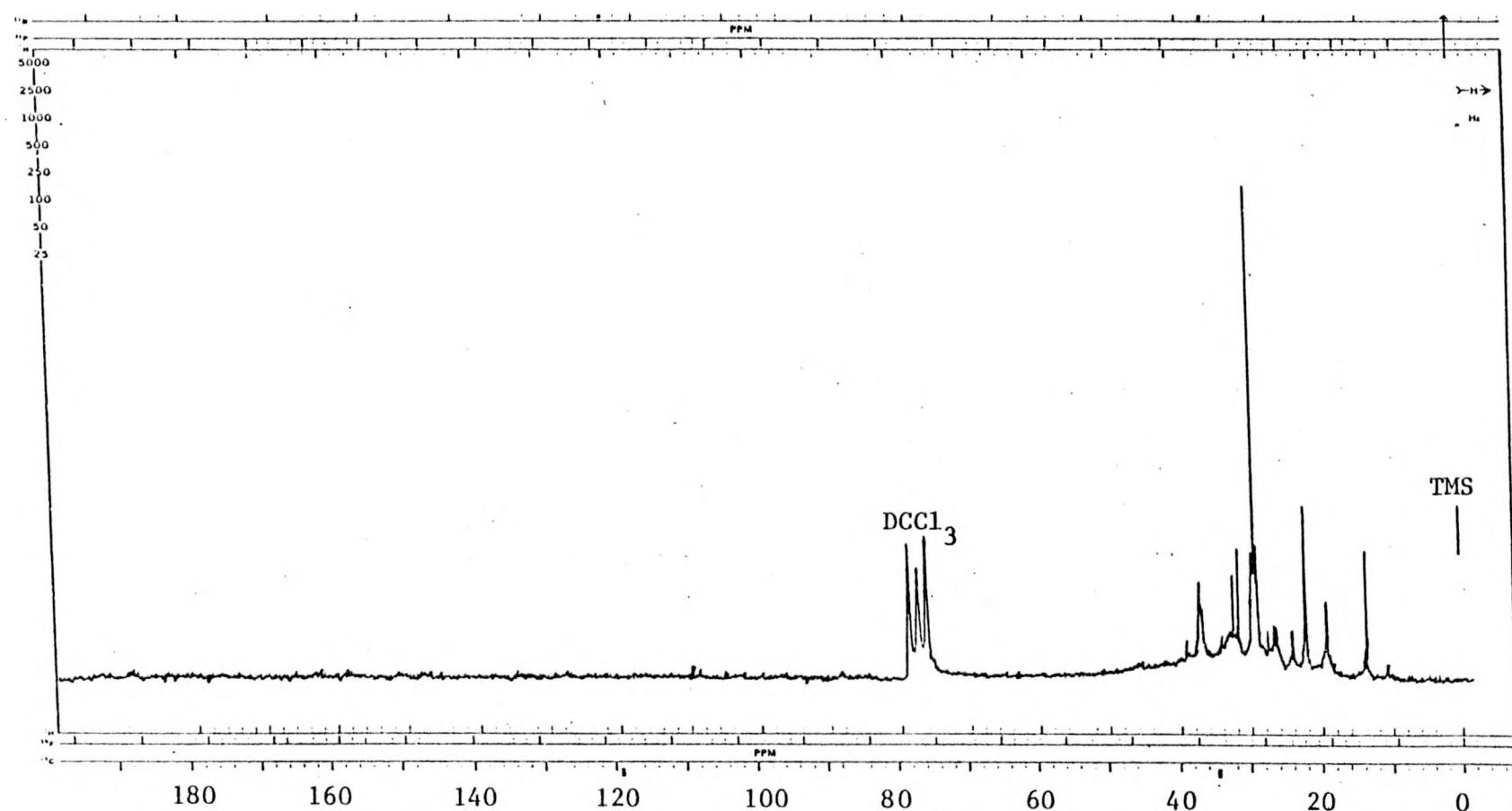
Gated Decoupled (off delay) Sample contained 0.05 M Cr(acac)<sub>3</sub>
