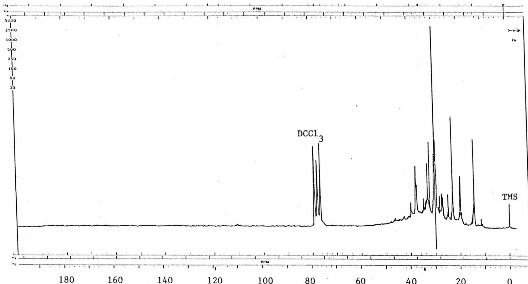
Gated Decoupled (off delay) Sample contained 0.03 M Cr(acac)<sub>3</sub>
