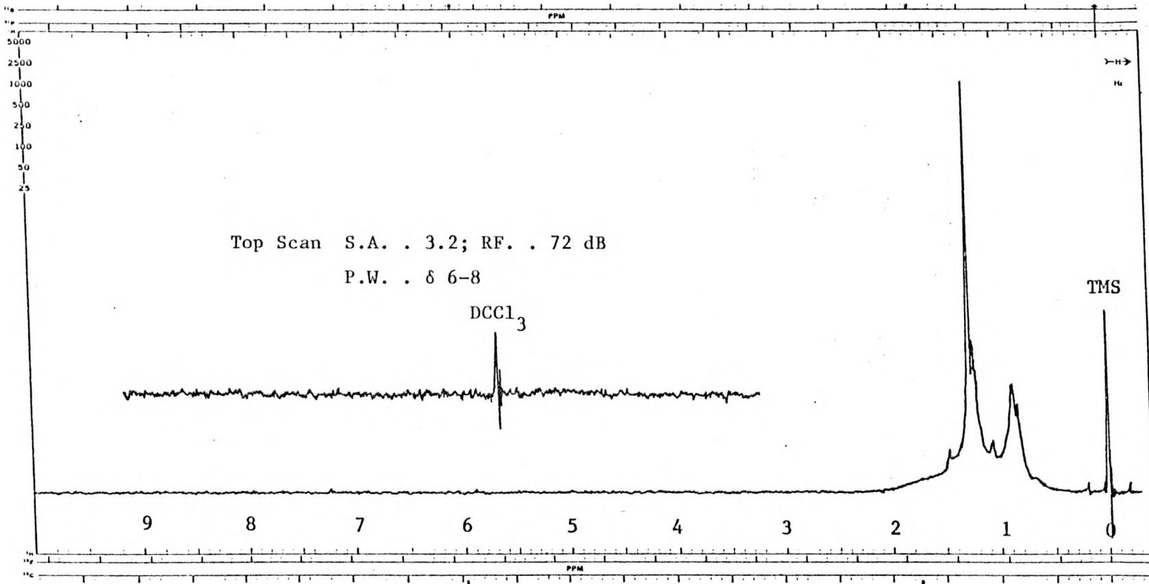
PFT CW X; Solvent. . DCCl<sub>3</sub> ; S.F. . 100.1 Hz; P.W. . 1000 Hz; F.B. . 2 Hz; Acq/S.A. . 1.0
