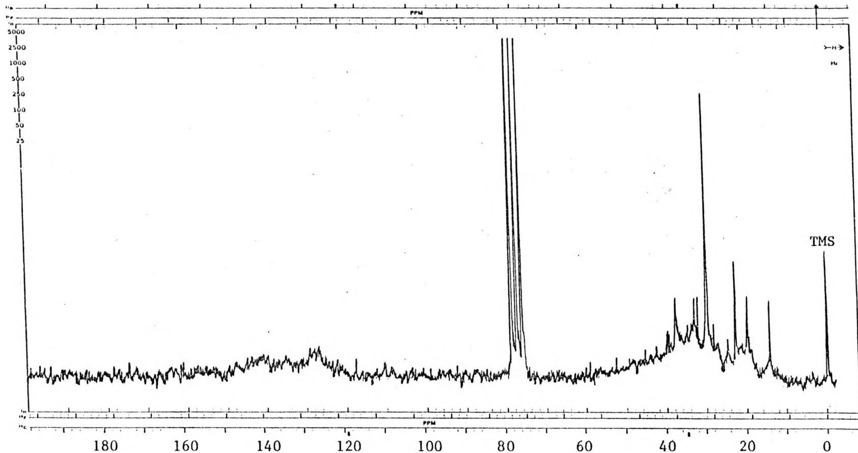
Gated Decouple (off delay) Sample contained 0.03 M Cr(acac)
