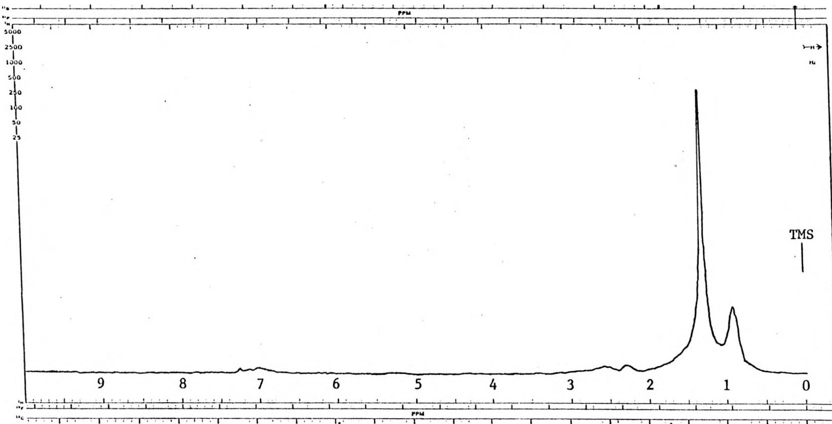
PFT X CW \_; Solvent. .  $\text{DCCl}_3$  ; S.F. . 100.1 Hz; P.W. . 1000 Hz; F.B. .  $\pm$  700 Hz; Acq/S.A. . 64
