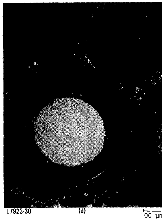
Fig. 4-23. Photomicrographs of fissile (small) and fertile (large) particles: (a) and (c) unirradiated; (b) and (d) irradiated in FSV fuel element 1-0743 to a fluence of 1.0 \times 10^{25} \text{ n/m}^2 ( E > 29 \text{ fJ} ) HTGR at a temperature of 720°C. (a) and (b) bright field illumination; (c) and (d) polarized light.
