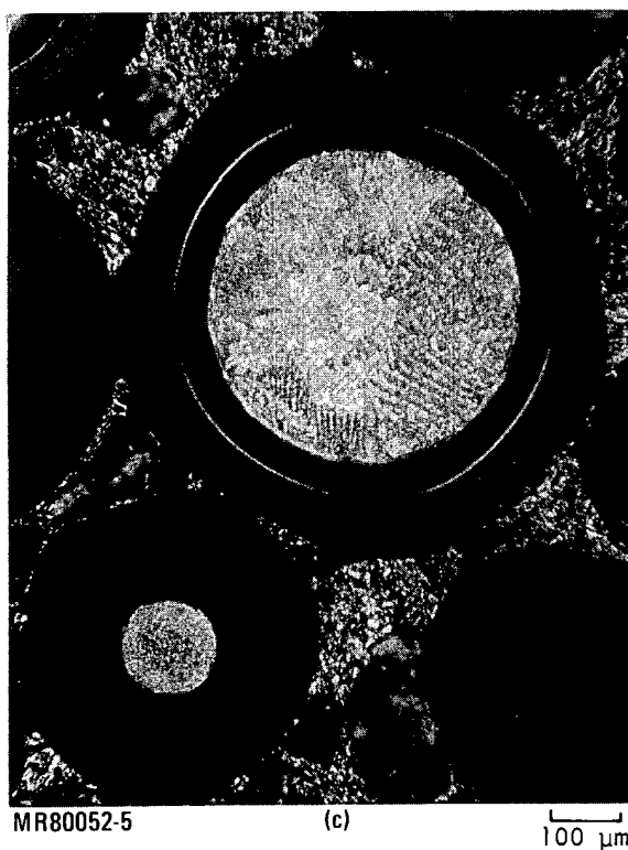
Fig. 4-23. Photomicrographs of fissile (small) and fertile (large) particles: (a) and (c) unirradiated; (b) and (d) irradiated in FSV fuel element 1-0743 to a fluence of 1.0 \times 10^{25} \text{ n/m}^2 ( E > 29 \text{ fJ} ) HTGR at a temperature of 720°C. (a) and (b) bright field illumination; (c) and (d) polarized light.
