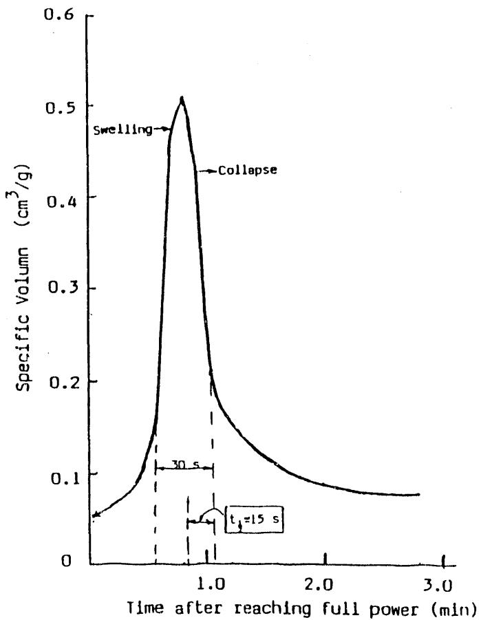
**Figure 4. Experimental Swelling/Foaming Behavior Noted for Previously-Irradiated U-metal Fuel Brought to Melt Temperatures.**
