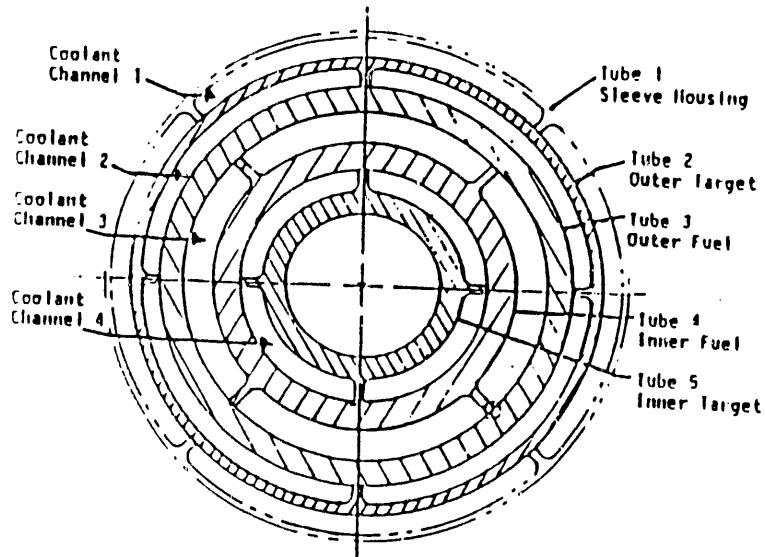
Figure 1. Illustration of Mark-22 Fuel/Target Assembly
