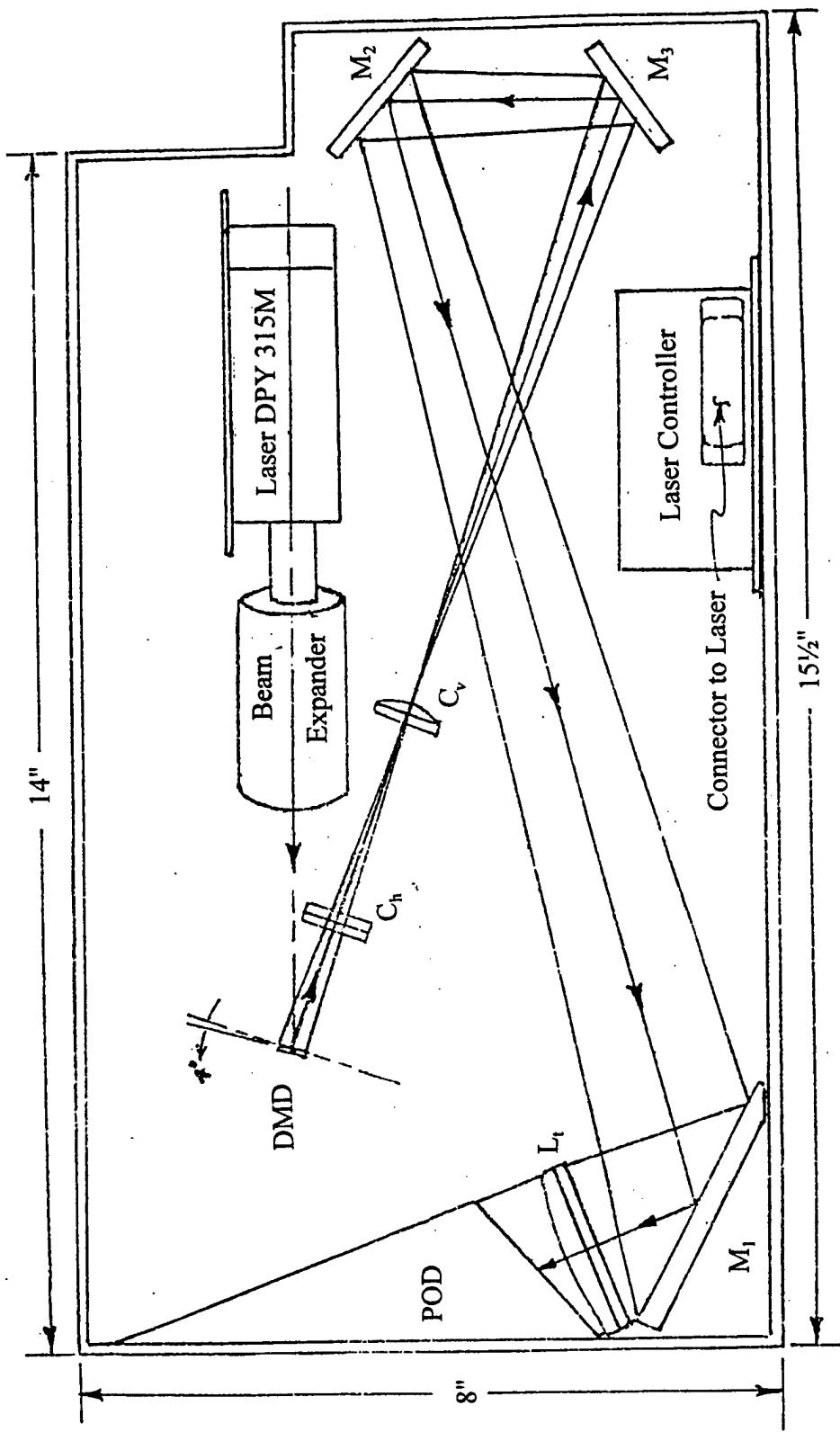
Figure 5 Packaging Design Layout -- Side View
