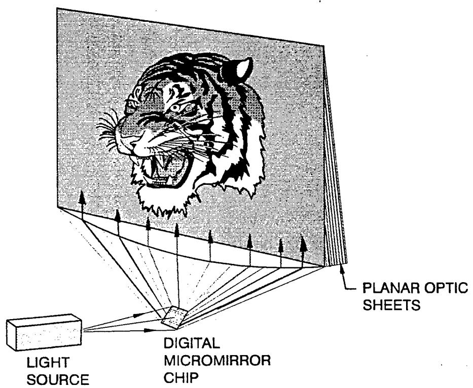
Figure 1 Functional Illustration of a Polyplanar Optic Display
