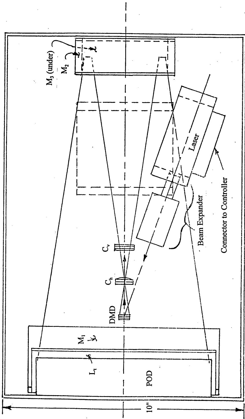
Figure 6 Packaging Design Layout -- Plan View
