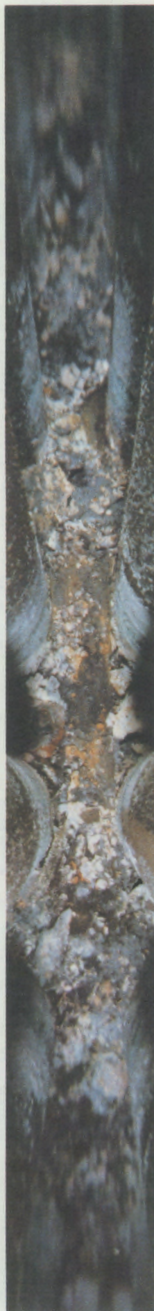
FIGURE 16. Photograph Taken With Tiny Lens Camera Looking Down at Tube Sheet Between Tube Rows
