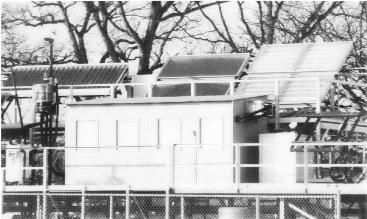
FIGURE 2.3 Collector Test Stand, Showing the Three Collector Arrays
