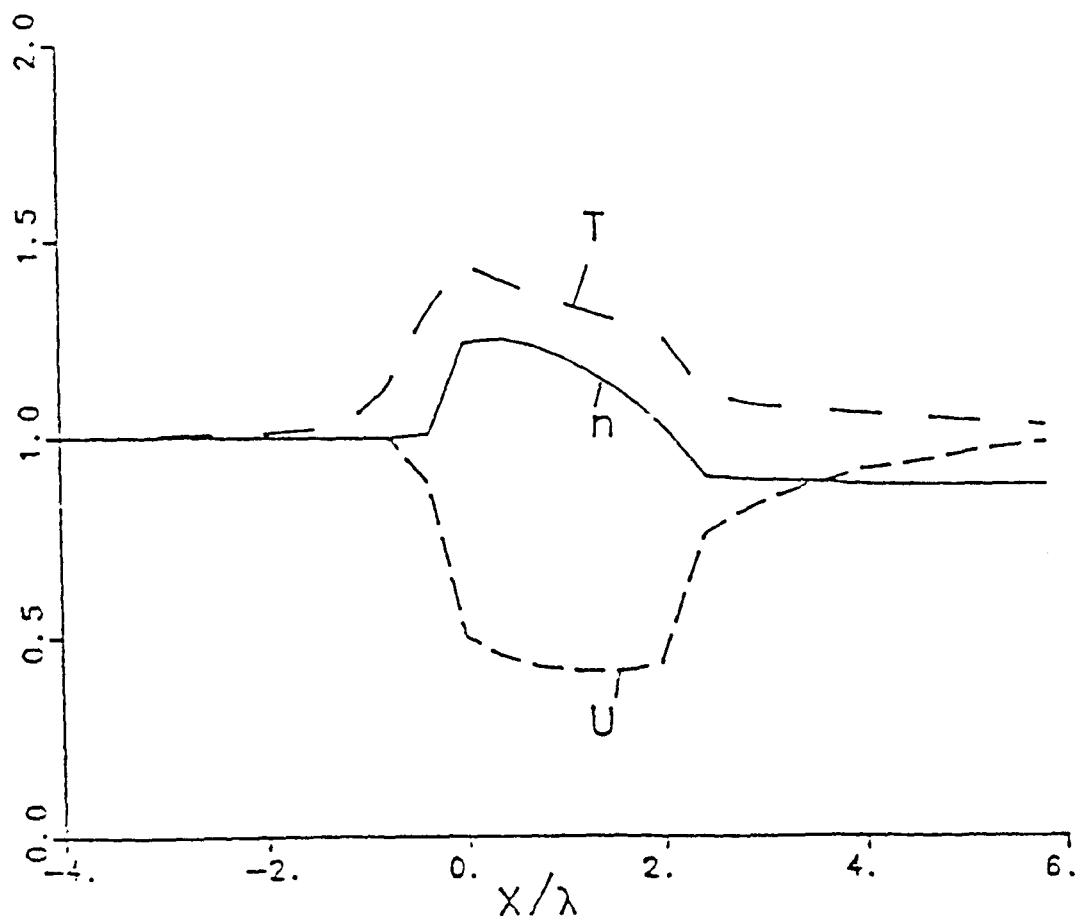
Fig. 6 Variation of density, mean velocity, and temperature along  $y = 0$ , for flow over a flat plate shown in Fig. 5. The plate extends from  $x = 0$  to  $x = 2$ . All fluid properties have been normalized by the corresponding freestream values.
