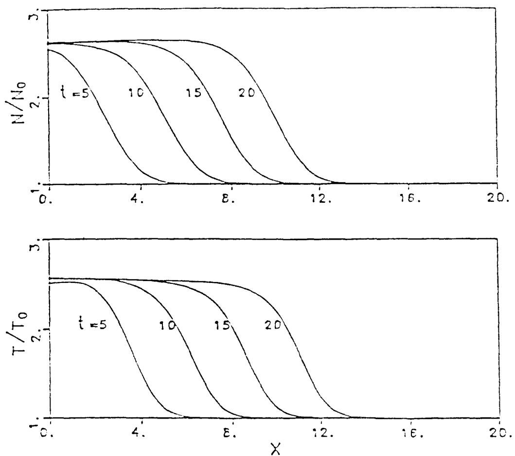
Fig. 2 Nondimensional density and temperature at various times for the reflecting piston problem when  $\text{Kn} = 0.02$ .
