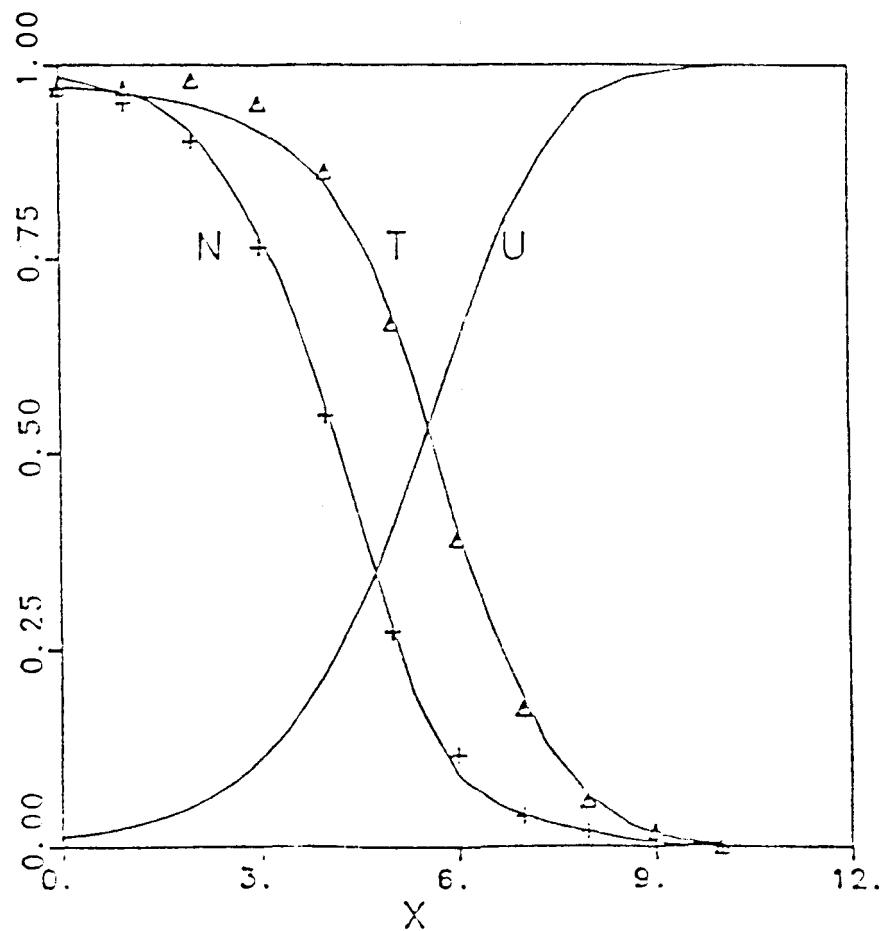
Fig. 1 Structure of a stationary shock wave in a hard-sphere gas at Mach 2.5. The solid lines are the results of this work; the symbols were taken from Aristov and Cheremisin.<sup>4</sup> N, U, and T denote reduced density, velocity, and temperature, respectively. X has been scaled by the mean free path in the unshocked gas.
