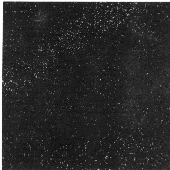
(c) TELLURIUM DISTRIBUTION AT 500X
