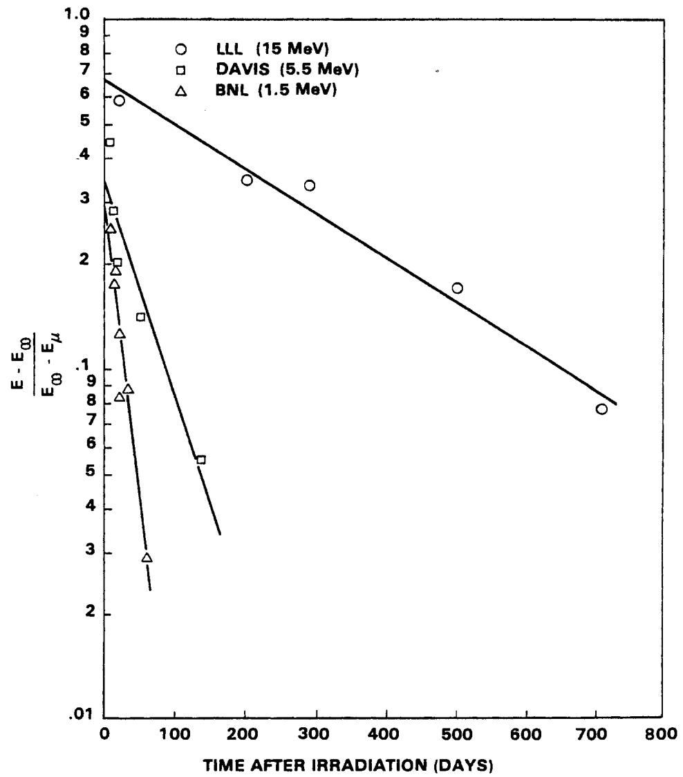
Figure 1. Change of Shear Modulus with Time.
