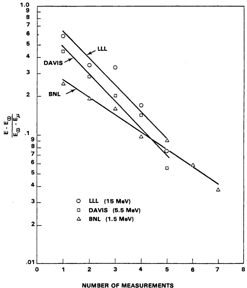
Figure 2. Change of Shear Modulus with Number of Measurements.
