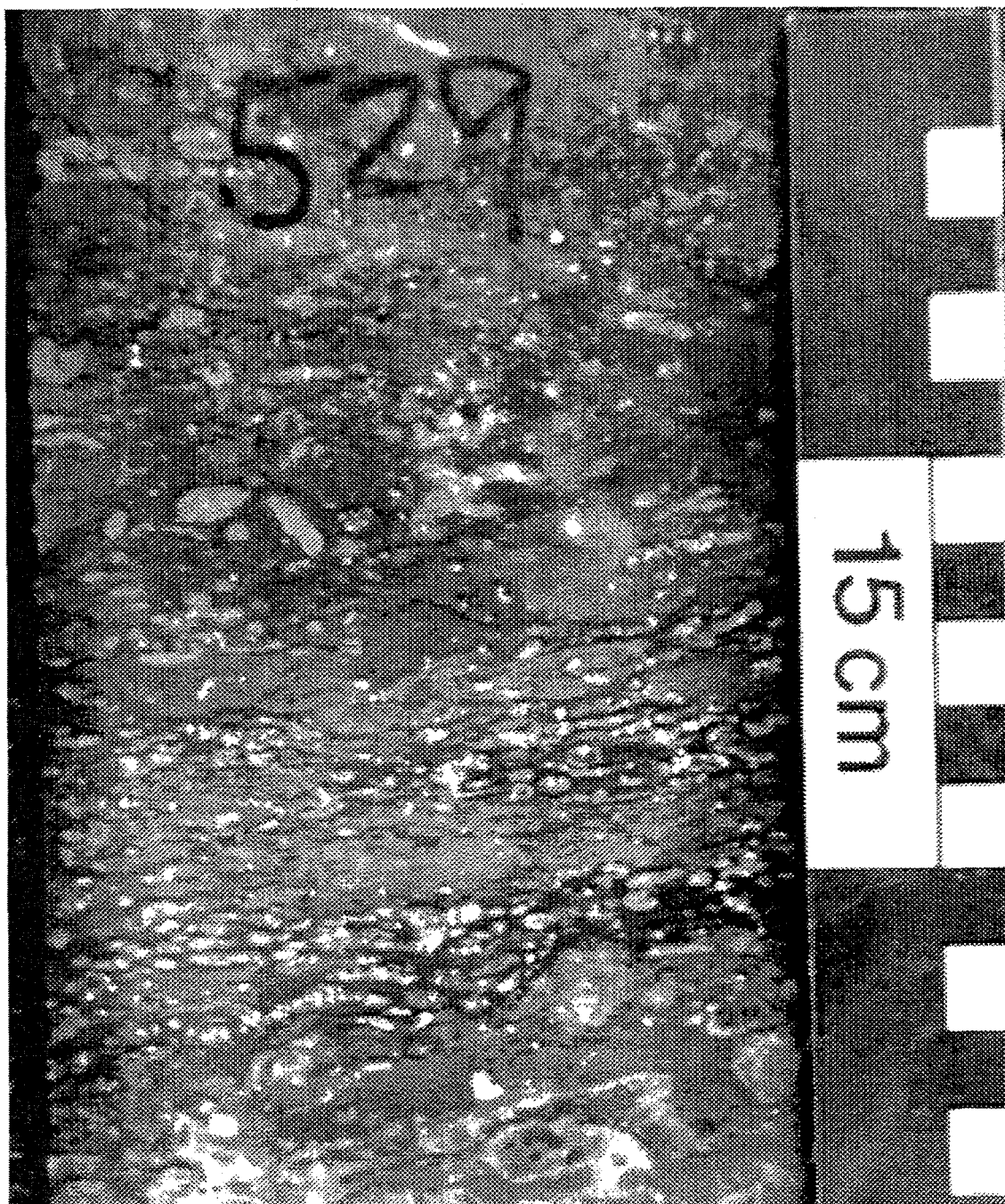
Figure 29: Core photo of D zone kerogenite beds and skeletal limestones. Shaley beds (Facies 1) are common in the Red River D porosity interval and are organic rich "kerogenites" (middle and base of sample). These sediments accumulated during sea level high stand or deepening events. Interbedded with these shales are skeletal lime mudstones and wackestone which were deposited in normal marine environments (Facies 2).
