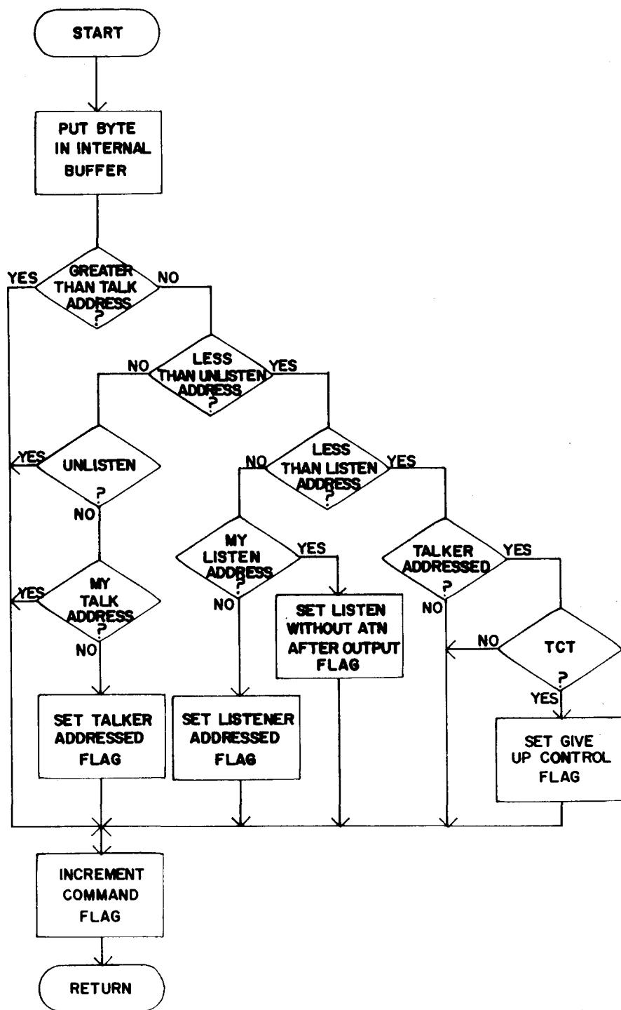
Figure 10. Save byte of bus command (SVBYTE).
