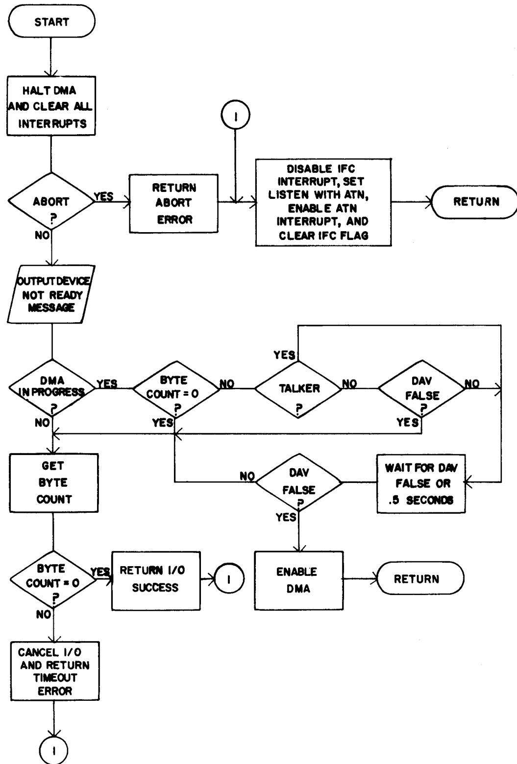
Figure 2. Device timeout (GPOUT).
