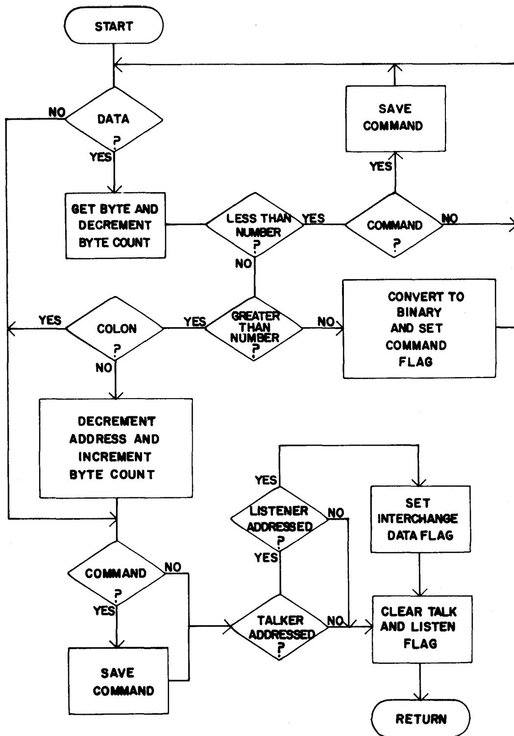
Figure 9. Convert bus command to binary (CNVB).
