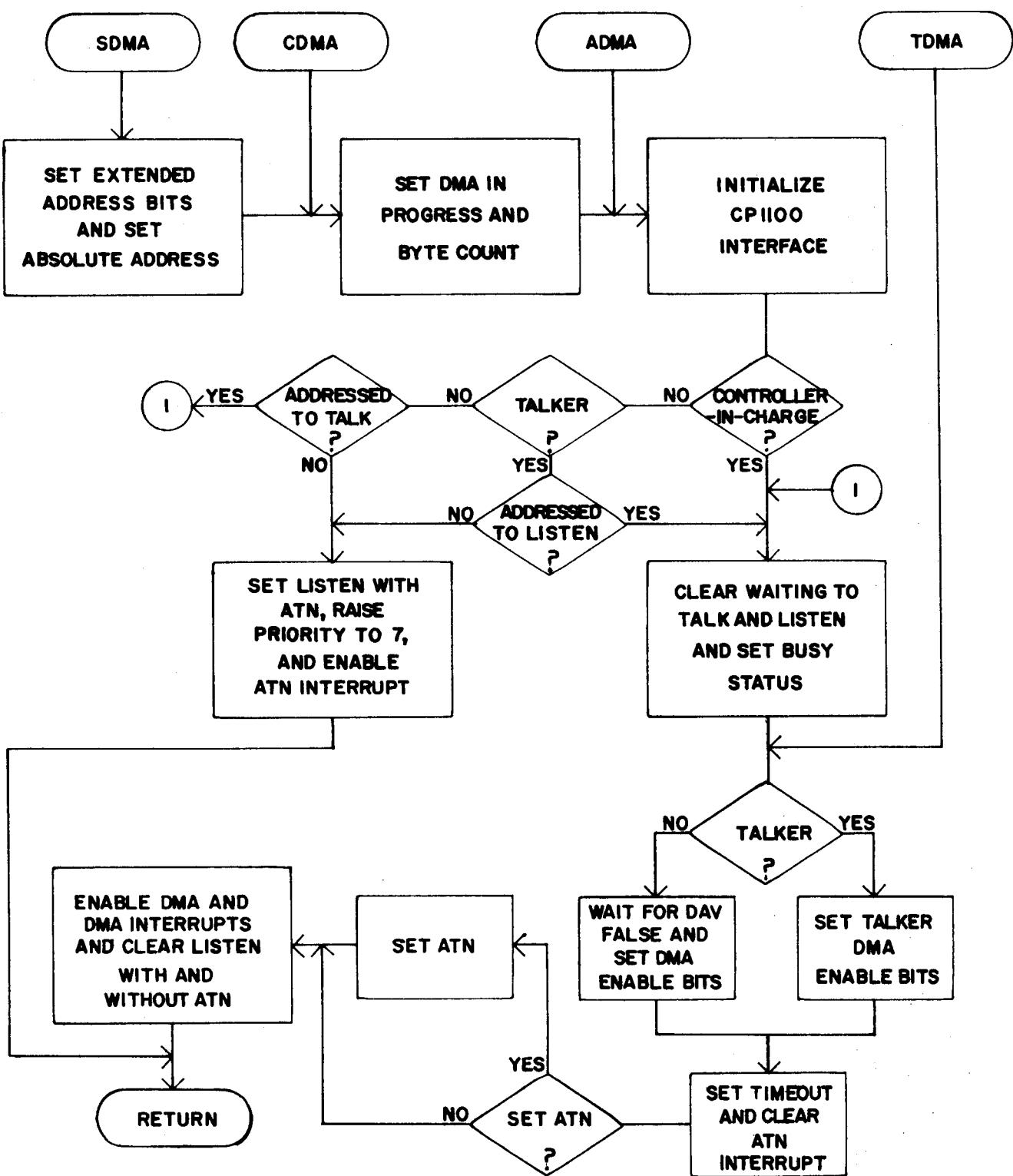
Figure 8. Enable DMA (SDMA, CDMA, ADMA, and TDMA).
