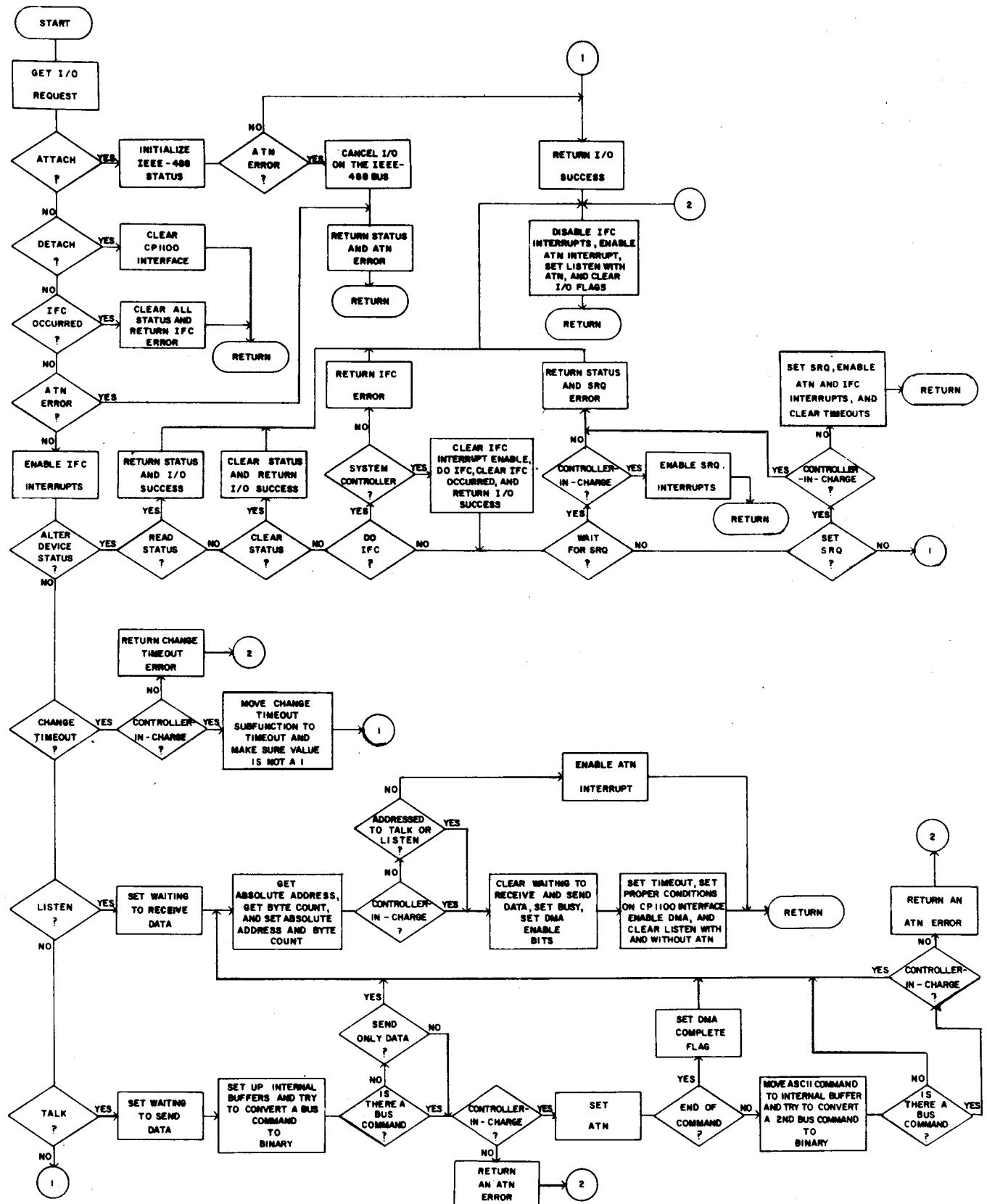
Figure 1. Device initiator (GPINI).
