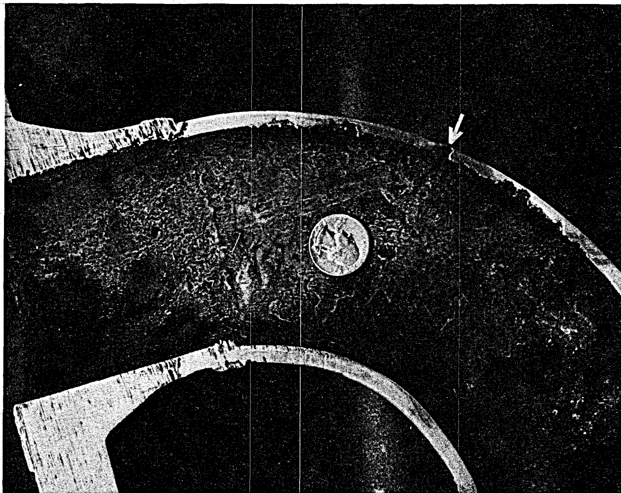
FIGURE 20. - Cross section of 3-inch elbow removed from input brine line showing erosion and pitting corrosion, 1976-77.
