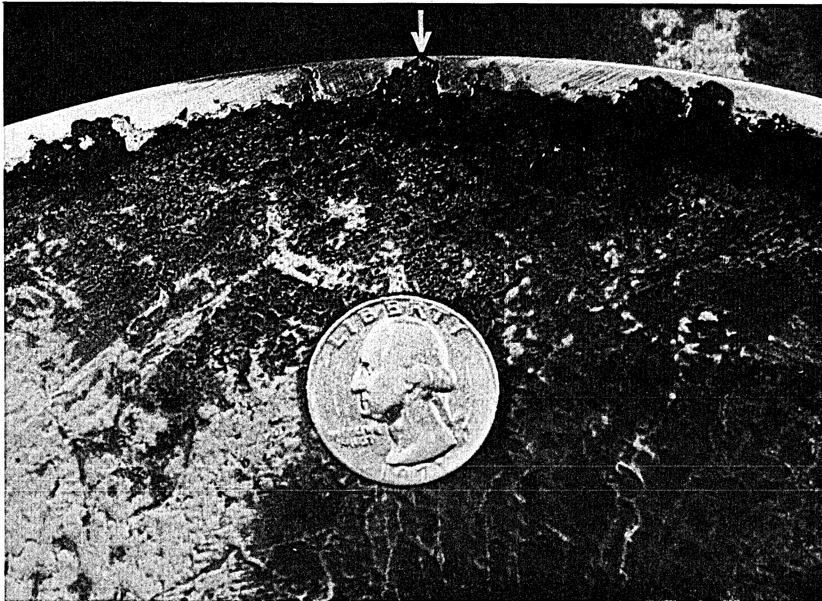
FIGURE 21. - Detail of pitting failure in 3-inch elbow, 1976-77.
