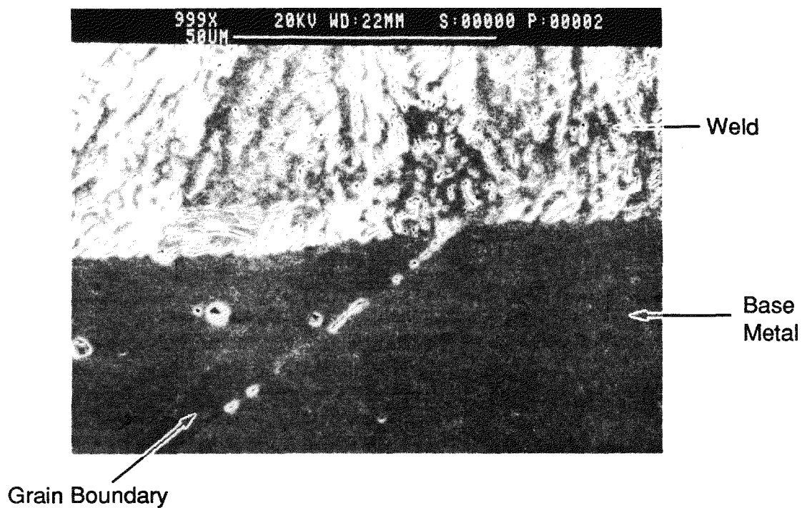
FIGURE 5. Scanning Electron Micrograph of Cavities on a Grain Boundary Adjacent to a Low Heat Input Overlay with 17 Appm Helium (Magnification = 1000X)
