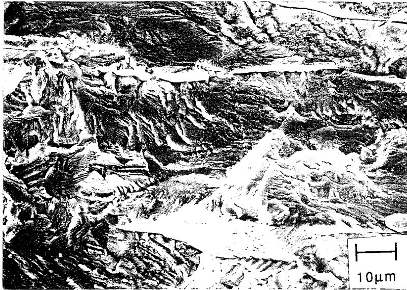
Fig. 4.36 Fracture surface of 0.5%ZrC fatigued in hydrogen gas at \Delta K=21 \text{ MPa}\sqrt{\text{m}} showing cleavage and fibrous tearing.
