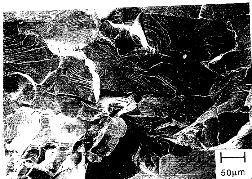
Fig. 4.32 Fracture surface of the ternary alloy fatigued in vacuum at \Delta K=30 \text{ MPa}\sqrt{\text{m}} showing cleavage and IG facets.
