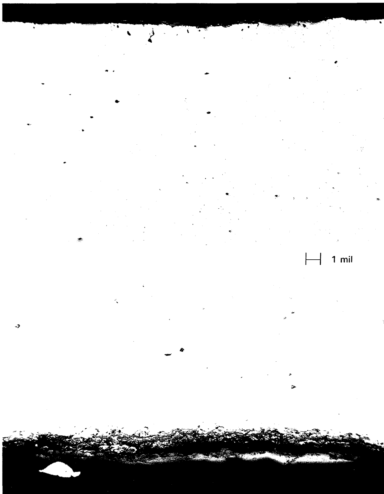
Fig. 22. One mil of internal oxidation was observed on the OD of 690-17 (top). The ID attack of the lean stainless steel can be seen in the bottom photomicrograph.
