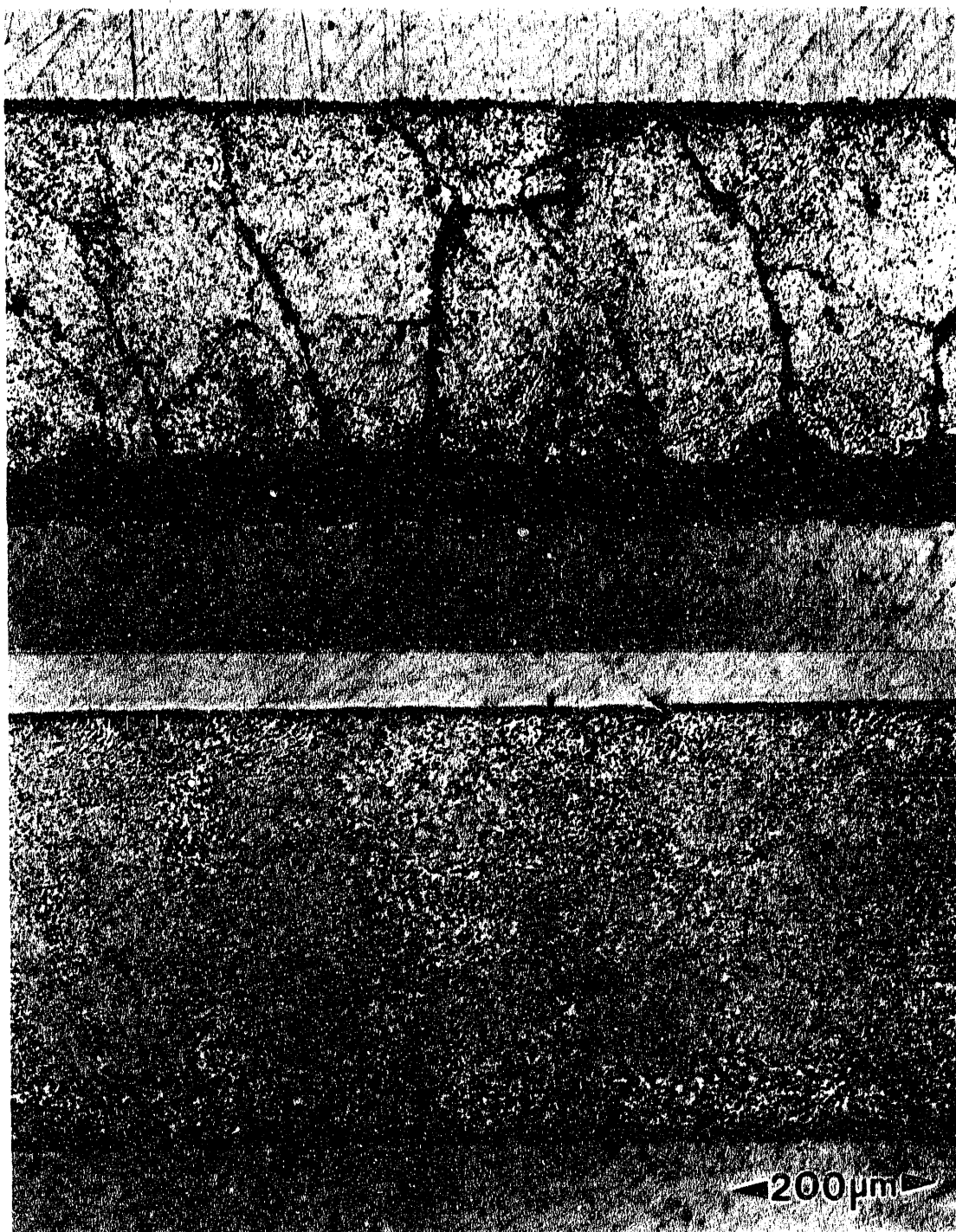
Figure 18. Optical micrograph of a polished solder joint deformed in shear. (top) The surface relief that develops with deformation. The deformation is localized to a thin band near the Cu/solder interface and along colony boundaries elsewhere in the joint. (bottom) The same specimen as in (top), but polished to remove the surface relief. There is an exact correspondence between the location of the major deformation band and a band of recrystallized and coarsened microstructure. The deformation elsewhere in the joint corresponds to the irregular material at the colony boundaries. The light regions are the Sn-rich phase, the dark regions are the Pb-rich phase. XBB887-7084
