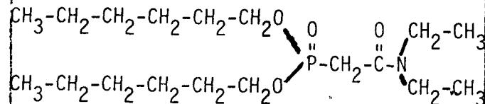
A new extraction chromatography process has been developed at RF for americium purification. The key to the process is the selective extraction of americium by the bifunctional organophosphorus extractant DHDECMP. The CMP extractant is sorbed on a solid support, Amberlite XAD-4, so that ion exchange columns can be used.
