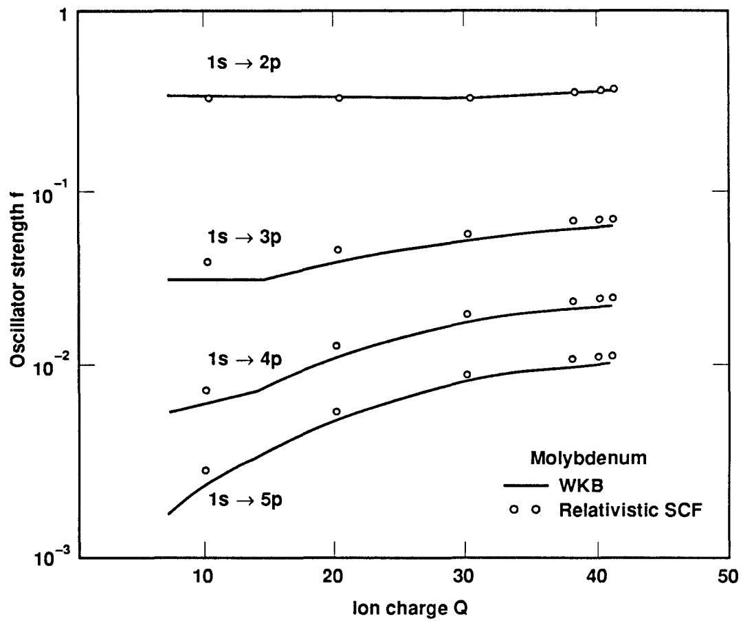
Figure 1. Oscillator-strength for transitions  $1s \rightarrow np$  of Molybdenum ions calculated by the method of Eq. (3). The comparison data was provided by D. A. Liberman and is obtained from a relativistic self-consistent field calculation.
