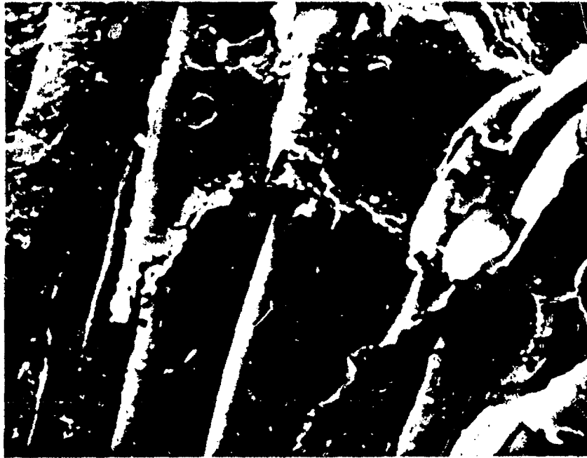
Figure 15. Scanning electron micrographs of 91-25 (high-Fe) oxidized in H_2O to 53.20% burn-off showing gross pitting and rough edges. (800X)
