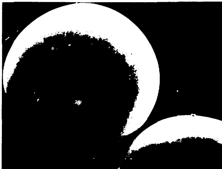
Fig. VII 15. Electroless plated nickel on GMB, first metallized with MO.C and activated with CVD nickel. (300X).
