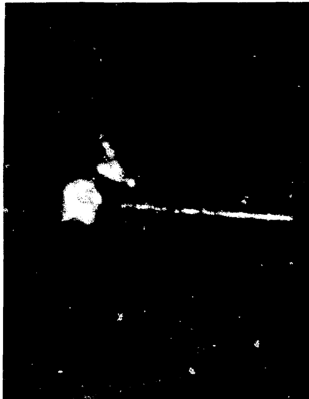
Fig. IV-24. Pinhole photograph of an imploded plastic-coated nickel shell backlit by radiation from a titanium source.
