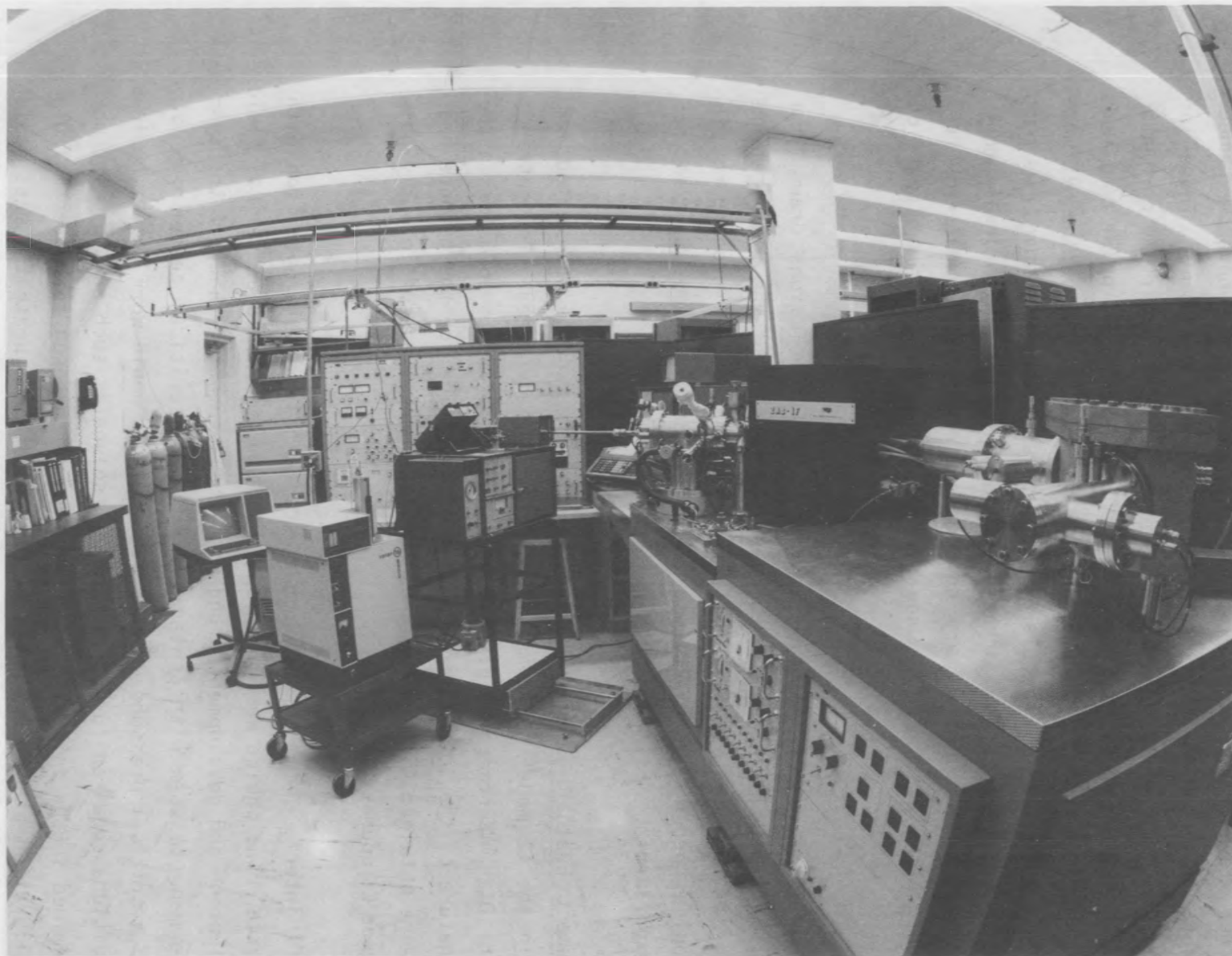
FIGURE 6. Photograph of the Assembled Direct Fluid Injection/Supercritical Fluid Chromatography/Mass Spectrometry Instrumentation, Showing the Interface Probe Ready for Insertion Into the Mass Spectrometer
