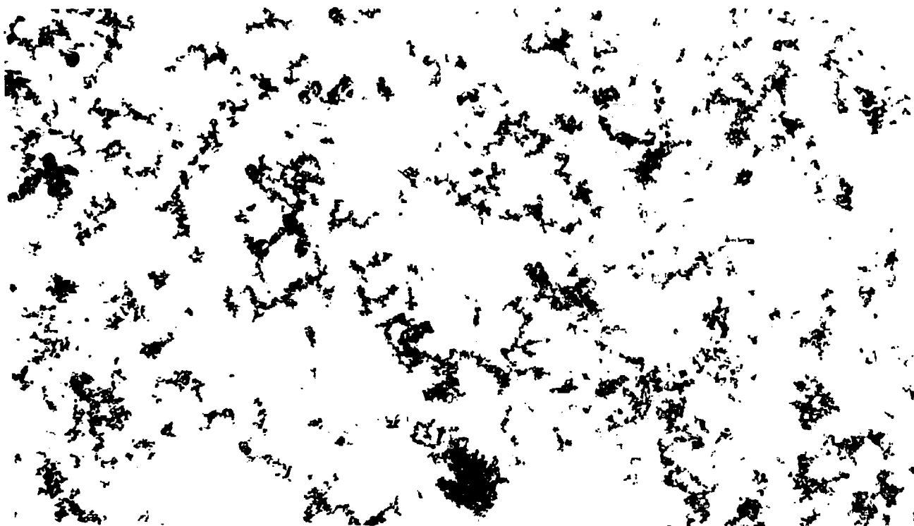
Fig. 9a. Photomicrograph of arc furnace \text{UO}_2 aerosol agglomerates at 5000X.
