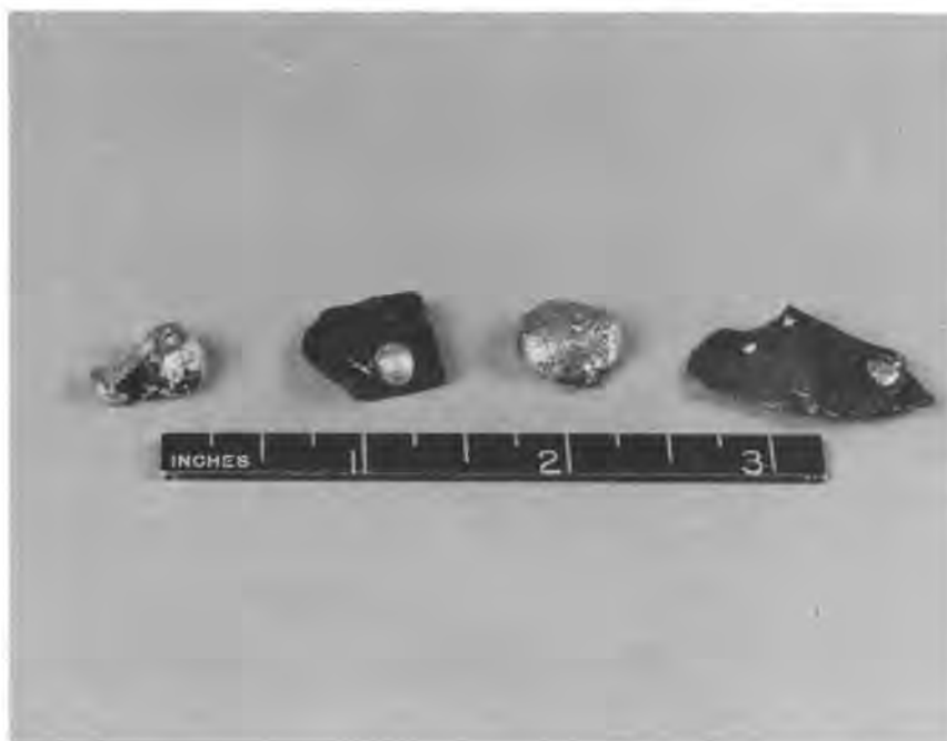
FIGURE 4. Metallic Buttons Removed from Bottom of Canisters 172 and 174
