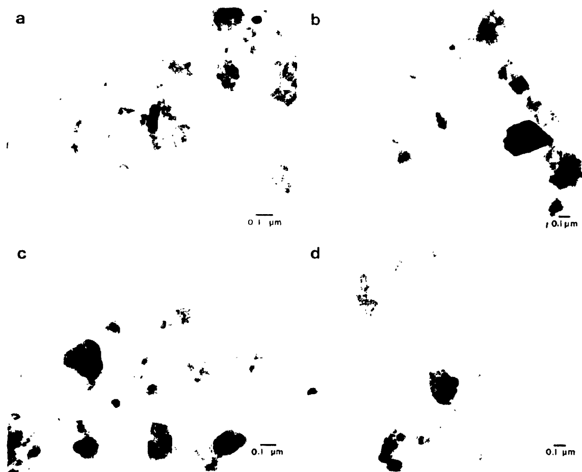
Fig. 11. Transmission electron micrographs of the clay fractions ( <2 \mu\text{m} ) from samples (a) A-5, (b) A-9s, (c) A-9d, and (d) A-16.
