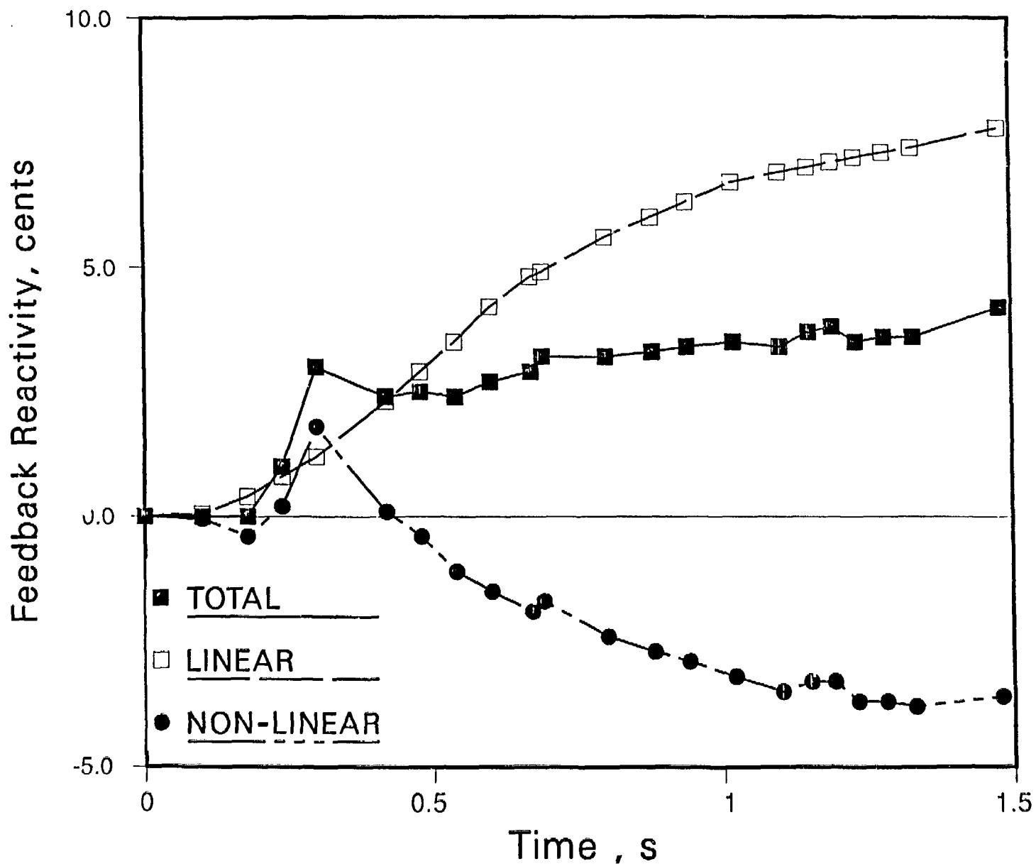
Fig. 3. Total Feedback Reactivity, Estimated Linear Feedback Reactivity and Deduced Non-linear Feedback Reactivity for a  $\sim 21$  Cent Control Rod Drop in Run 143A.
