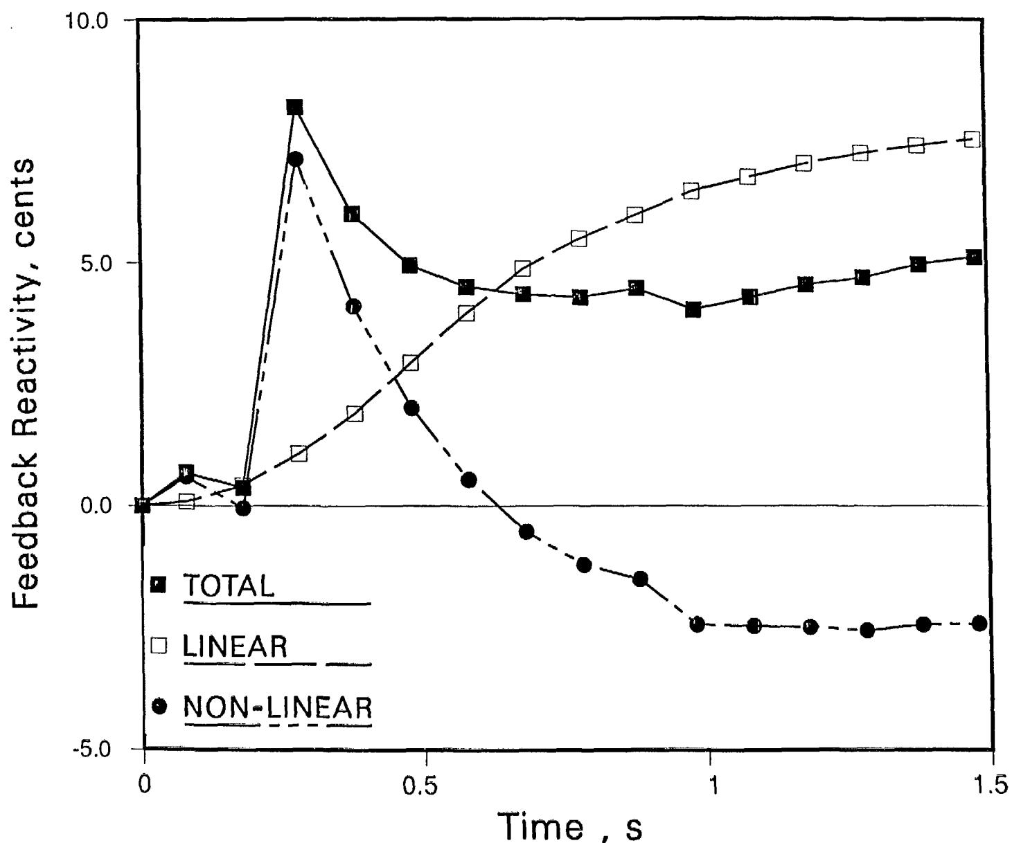
Fig. 2. Total Feedback Reactivity, Estimated Linear Feedback Reactivity and Deduced Non-linear Feedback Reactivity for a  $\sim 21$  Cent Control Rod Drop in Run 130A.
