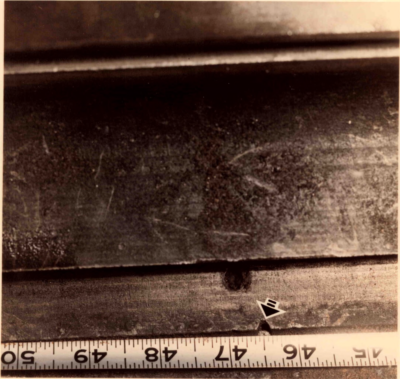
Fig. 7. Gear Tooth Notch in Lathe Bed
