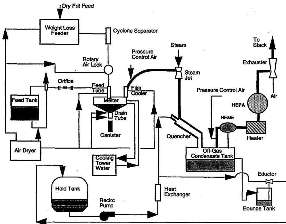
Figure 1. Am/Cm Melter 2A bushing melter pilot system schematic
