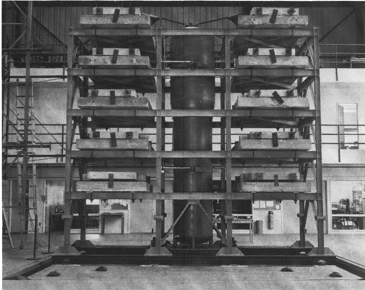
FIGURE 2 MODEL MOUNTED ON THE SHAKING TABLE AT EERC
