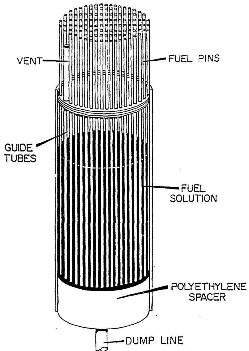
FIGURE 1. Schematic of Boiler Tube-Type Tank
