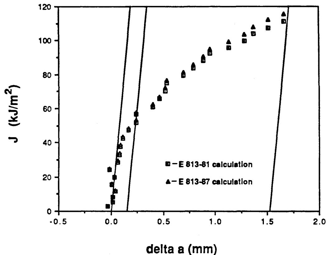
Figure 2.  $J$  versus crack growth behavior for a typical sample as calculated by the two versions of ASTM E 813. [Sample 1U,  $B_{\text{net}} = 20.6 \text{ mm}$ ,  $W = 50 \text{ mm}$ , temp. =  $25^\circ\text{C}$ ]
