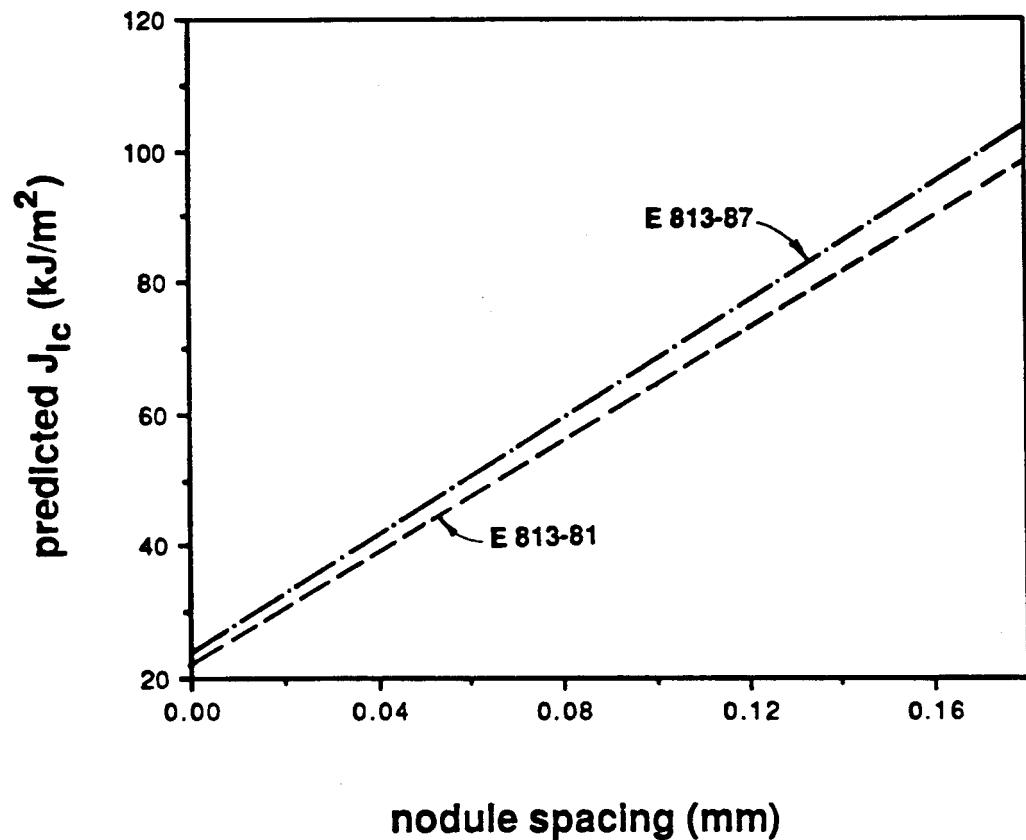
Figure 8. Comparison of the linear regression fit of the fracture toughness for the set of DCI alloys in which the  $J_{Ic}$  values were determined by the two versions of the ASTM E 813.
