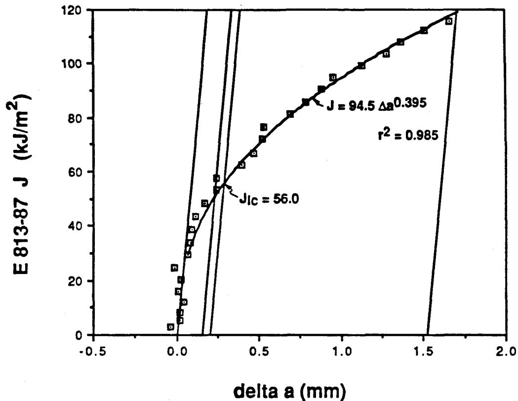
Figure 4. Power law fit of the valid  $J$ - $\Delta a$  data, and determination of  $J_{Ic}$ , according to ASTM E 813-87. [Sample 1U,  $B_{net} = 20.6$  mm,  $W = 50$  mm, temp. = 25°C]
