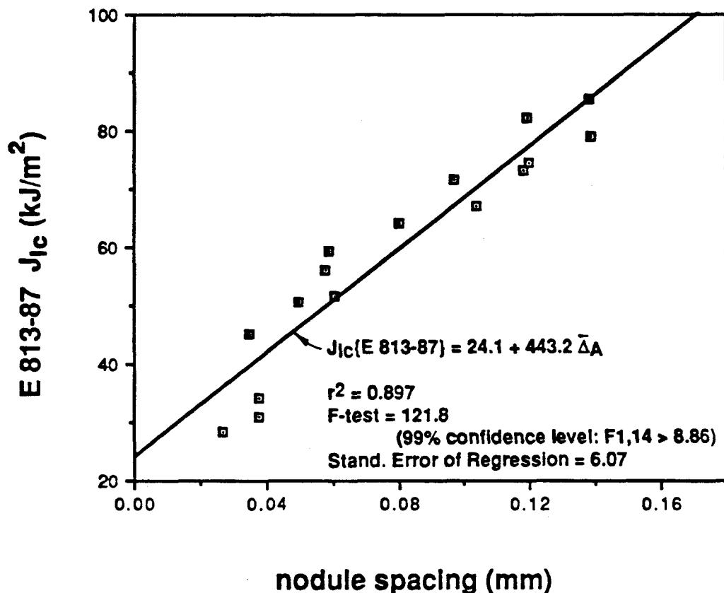
Figure 7. Results of the linear regression fit of the  $J_{Ic}$  data (calculated to the revised version: E 813-87) for the set of DCI alloys, showing the fracture toughness related to average graphite nodule spacing (determined by a two-dimensional measurement).
