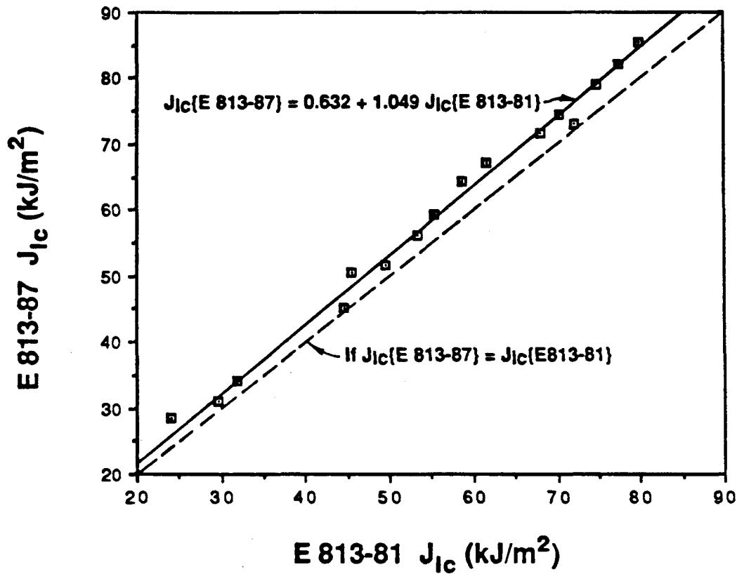
Figure 5.  $J_{Ic}$  determined by the new version (E 813-87), plotted against  $J_{Ic}$  as calculated by the original version (E 813-81) for the set of ferritic DCI alloys.
