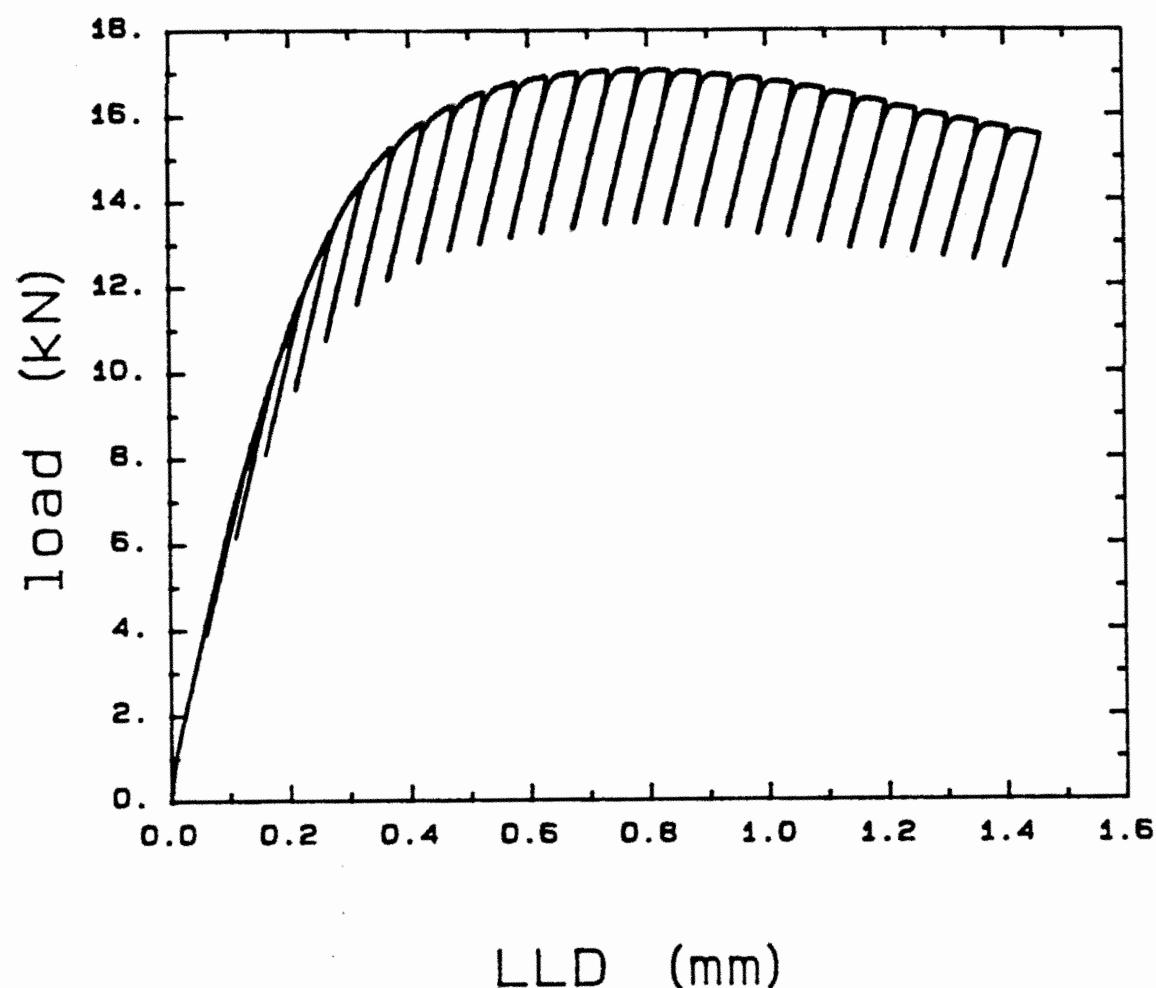
Figure 1. A typical load - LLD (load line displacement) record for a single specimen unloading compliance J-integral test (to either E 813-81 or E 813-87). [Sample 1U,  $B_{net}$  = 20.6 mm,  $W$  = 50 mm, temp. = 25°C]
