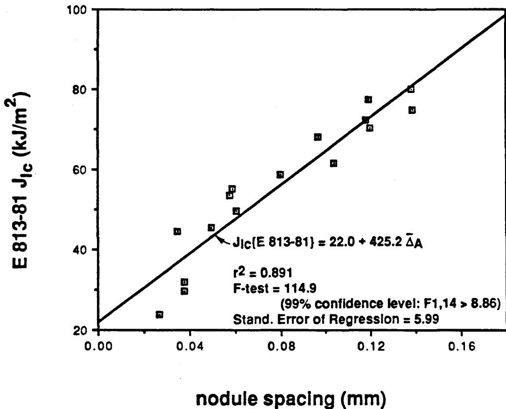
Figure 6. Results of the linear regression fit of the  $J_{Ic}$  data (calculated to the original version: E 813-81) for the set of DCI alloys, showing the fracture toughness related to average graphite nodule spacing (determined by a two-dimensional measurement).
