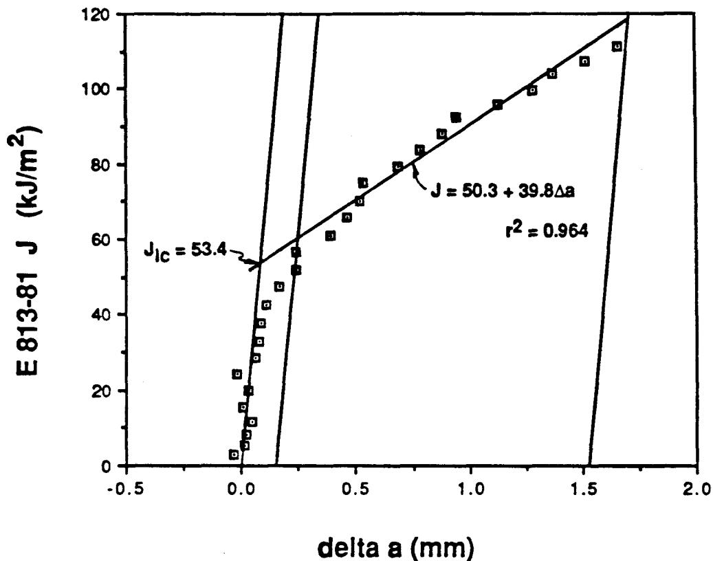
Figure 3. Straight line fit of valid portion of the  $J$ - $\Delta a$  data, and determination of  $J_{IC}$ , according to ASTM E 813-81. [Sample 1U,  $B_{net} = 20.6$  mm,  $W = 50$  mm, temp. = 25°C]
