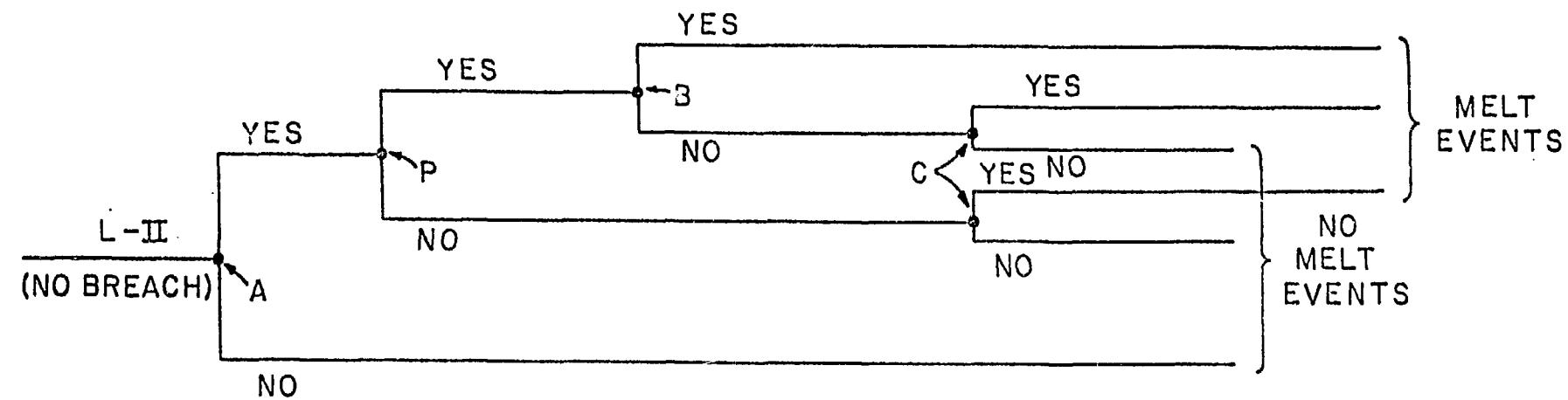
Figure 2: Event Tree for LOHS Scenarios for which there is not an Initial Breach of the PHTS Pressure Boundary.
