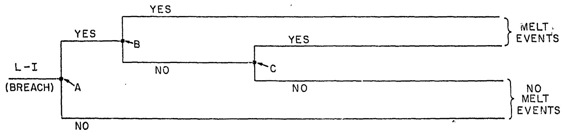
Figure 1: Event Tree for LOHS Scenarios for which there is an Initial Breach of the PHTS Pressure Boundary.
