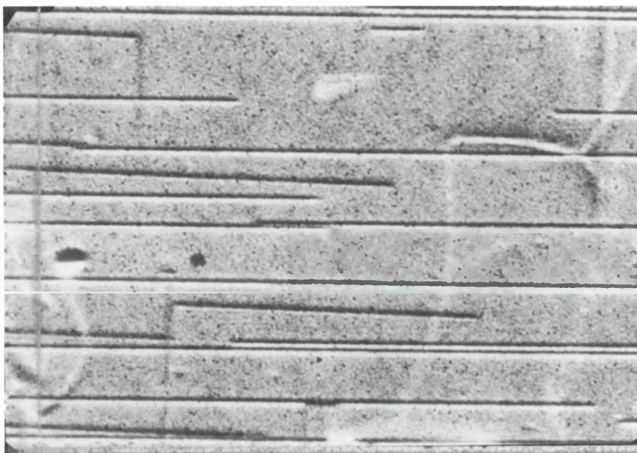
Figure 2 XRT showing dislocations that are bent at substrate/SLS interface.
