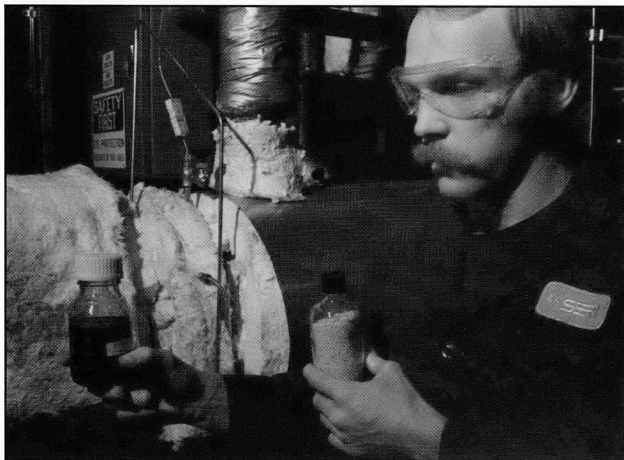
Engineers at the Solar Energy Research Institute have developed a fast-pyrolysis process to convert wood and municipal solid wastes to gasoline and other valuable chemicals.
