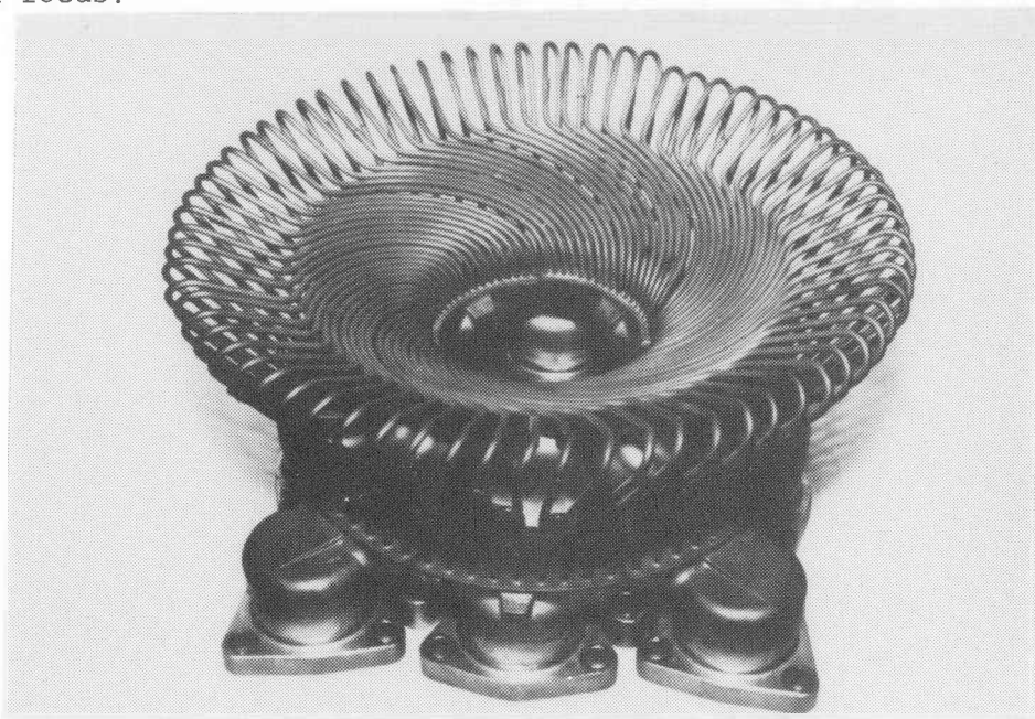
United Stirling ESOR-IIB heater head used on the Advanco Dish-Stirling Module. The oversized heater head tubes are spread out to improve the flux distribution and reduce thermal stress, but engine and receiver performance are compromised.
