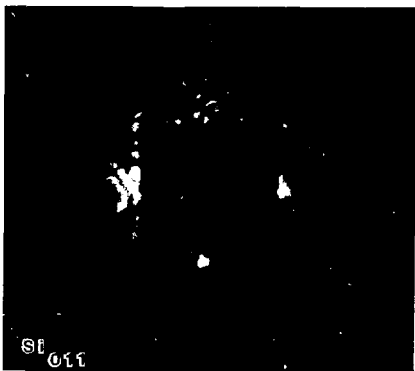
Figure 2-3. Convergent-beam electron-diffraction pattern from a Si specimen in the [011] orientation showing higher-order Laue-zone lines within the central disc. (XBB 836-5048)
