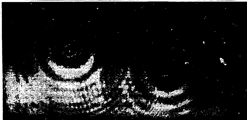
Figure 3. Digital reconstruction of the hologram shown in Figure 2. The depth of the plane of the reconstruction has been chosen to give the best correspondence to the image in Figure 1. Most of the features of the direct image are visible. The remaining interference rings are due primarily to the presence of the virtual image in the reconstruction. Improved reconstruction techniques and alternative holography geometries are being explored.
